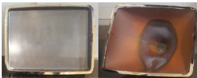
Figure 1. Left, front part cathode ray tube (CRT F ); right, rear part (CRT R ).
