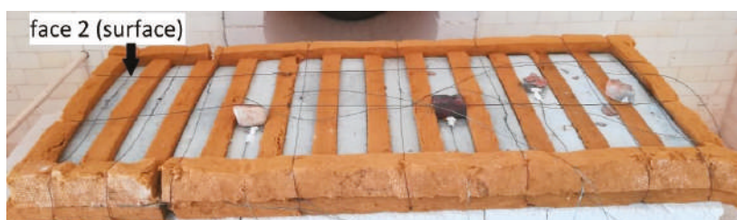
Figure 4. Set-up of specimens from Series B, C, D and F for the execution of the fire test. At the end of each fire test, the specimens were left to cool down naturally, without getting them out of the furnace before reaching the room temperature. The door of the furnace was only opened after the temperature had dropped to 180 °C, to avoid sudden cooling down which could harm the specimens and the furnace itself.
