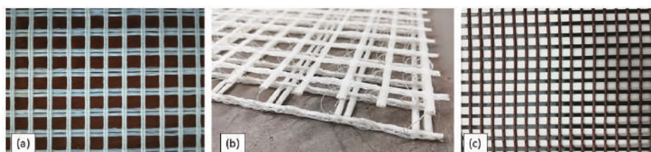
Figure 1. (a) 2D styrene-butadiene (SBR) coated glass-fiber textile; (b) 3D SBR coated glass-fiber textile; (c) SBR coated carbon-fiber textile.
