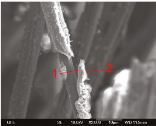
Figure 13. SEM image of unimpregnated carbon. 1 and 2 EDX analysis in the marked area.
