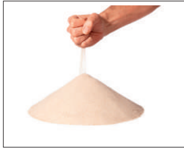
Figure 12.6 A marginally stable, forced-dissipative system. The angle of repose is maintained, on average, by random, small avalanches. Source: iStock/Getty Images
