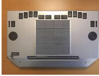
Fig. 2. The dot-matrix display used in the study
