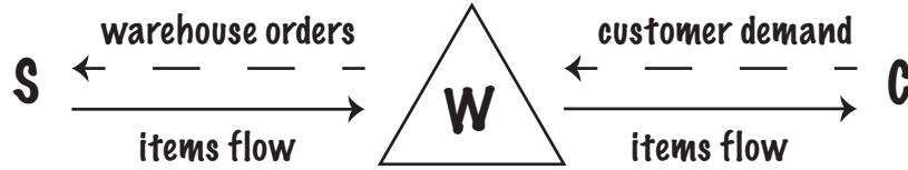
Fig. 5 A simple inventory system; physical flows and information flows are represented via solid and dashed lines, respectively.
