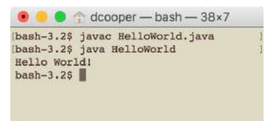
Figure 1.11: Compiling and Running the HelloWorld.java console application program.
