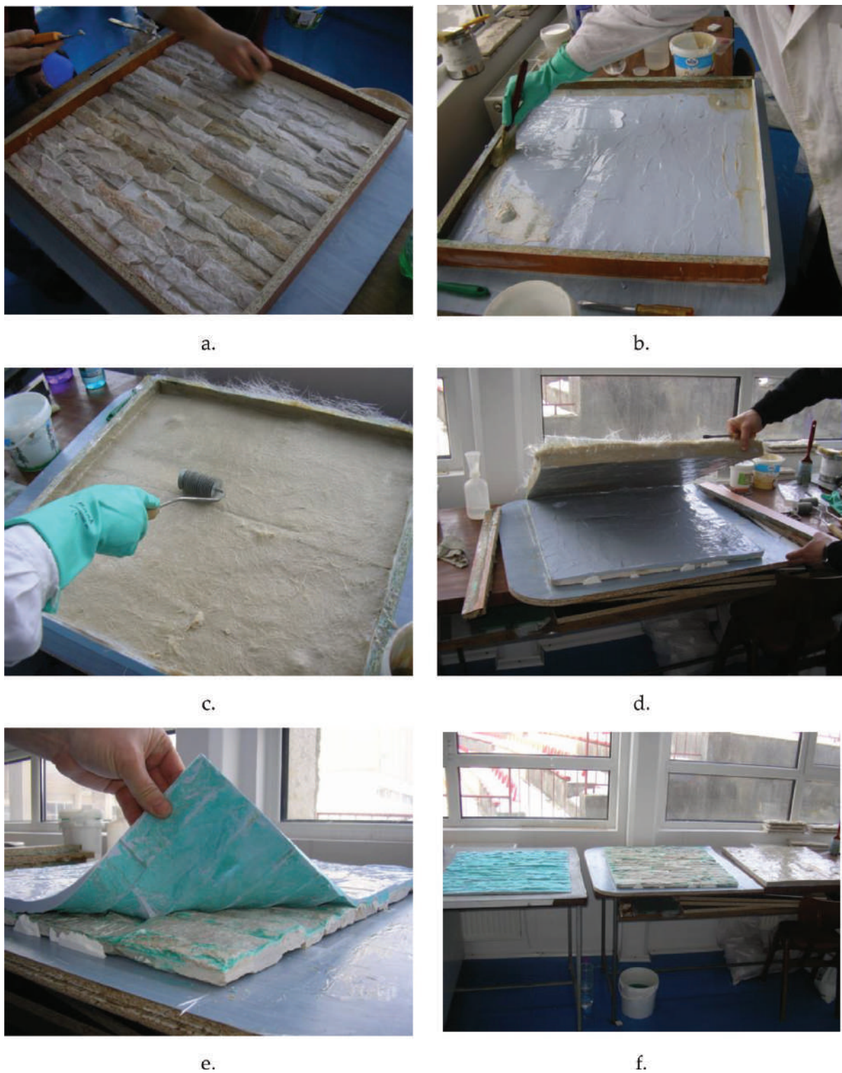
Figure 3. Steps of mold forming.
