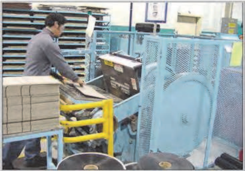
Fig. 24. Press Machine that cuts the BC Bags
