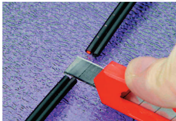
Figure 14. POF fiber cutting easy with cutter knife.
