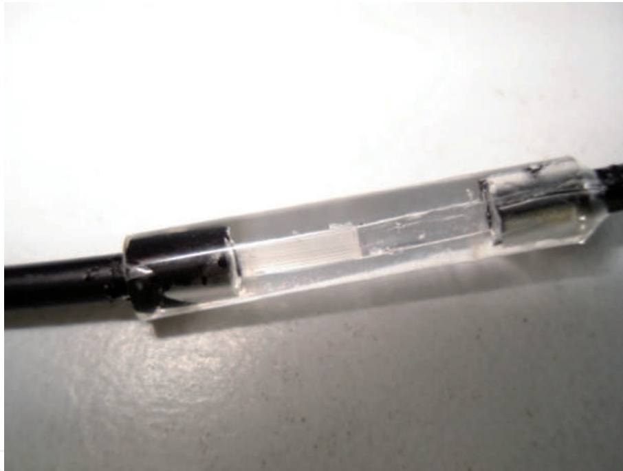
Figure 13. Optical splice with low attenuation.
