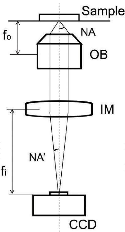
**Figure 1.** A diagram of an inverted microscope with an infinity-corrected optical system. OB, objective lens; IM, imaging lens; NA, numerical aperture of the objective lens;  $NA'$ , numerical aperture of the imaging lens;  $F_o$ , focal distance of the objective lens;  $F_i$ , focal distance of the imaging lens.
