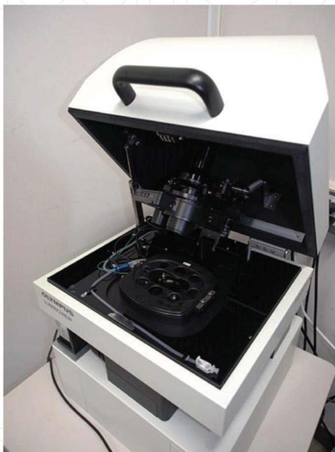
**Figure 5.** Bioluminescence microscope, LV200. A stage-top incubator with temperature and CO<sub>2</sub> gas controllers was added to the sample stage. The observation area was covered with a dark box.
