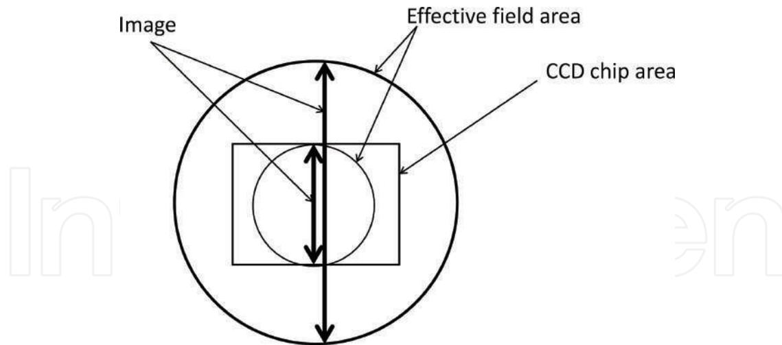
**Figure 4.** An effective field diagram on a CCD chip. Generally, the area of a CCD chip is smaller than the effective field area, and an image on a CCD chip is only some of light collected by the objective lens. If all light is collected on the CCD chip as an image by reducing the magnification using an intermediate tube lens or modified imaging lens, the light intensity of a pixel of the CCD chip increases.
