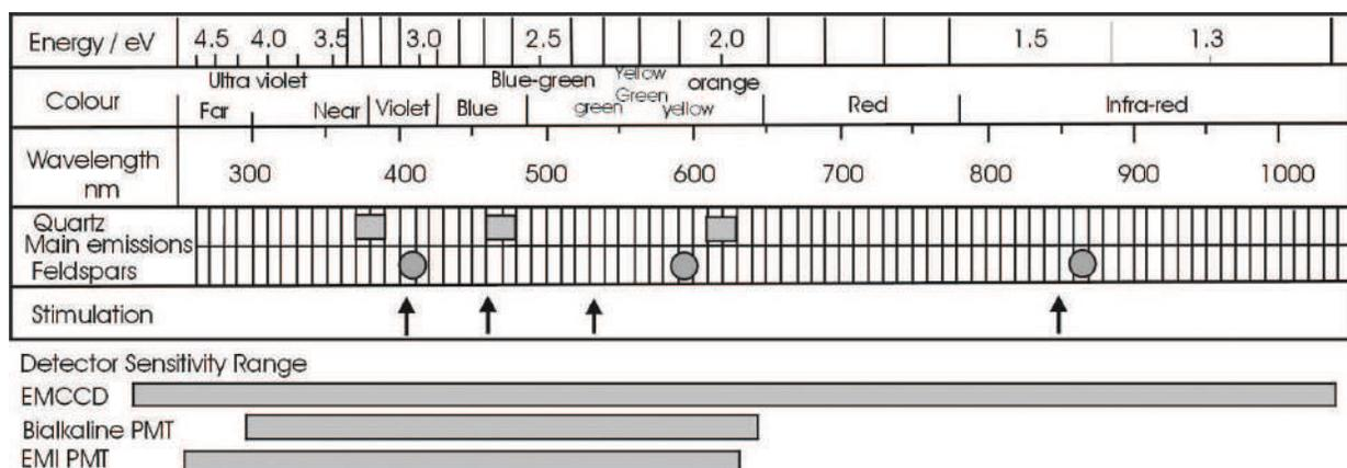
**Figure 7.** Main emission wavelengths for quartz and feldspars used in luminescence dating as well as wavelengths employed for stimulation. Sensitivity ranges for some detectors are also shown. Standard bialkaline photomultipliers (PMT) and EMI 9235QB PMTs do not detect emissions beyond 650 nm, whereas electron multiplying CCD (EMCCD) cameras can capture the whole range (modified after Ref. [54]).
