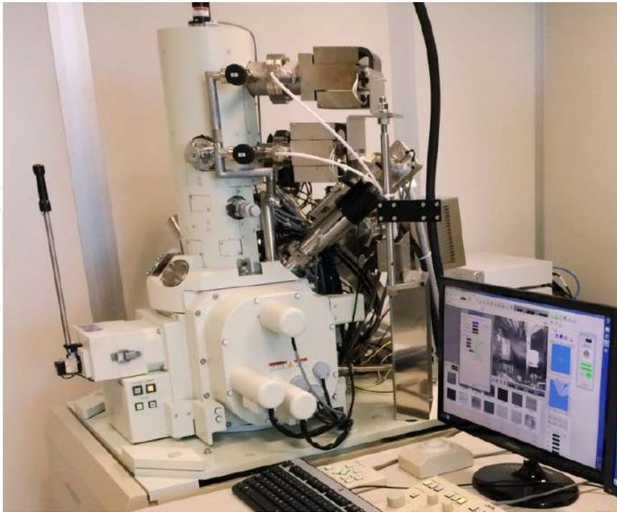
**Figure 2.** A commercial FIB/SEM workstation equipped with GIS, micromanipulator, and EDS detector (JEOL JIB 4601F MultiBeam System at Sabanci University Nanotechnology Research and Application Center-SUNUM)
