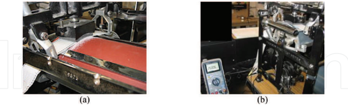
Figure 4. Abrasion testing on a white webbing with conductive yarns (a). A multimeter measured the change in resistance after successive series of abrasion cycles (b).
