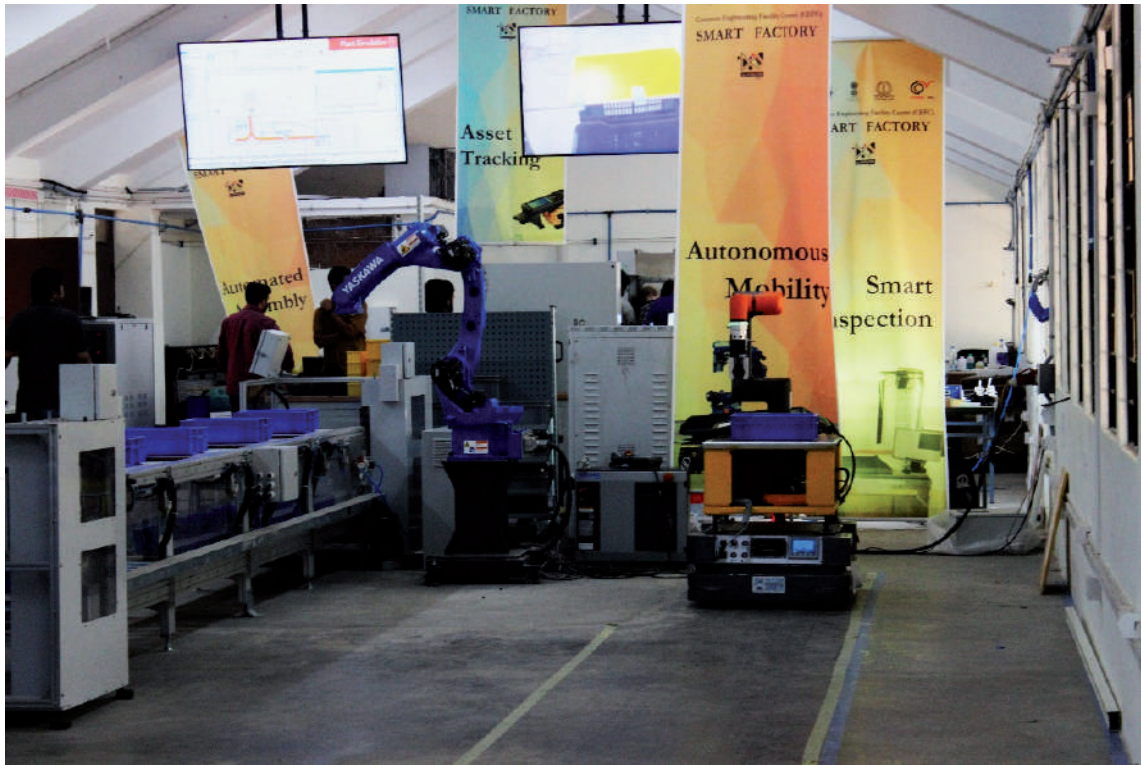
Figure 5. Autonomous mobile vehicle/Hanwha Cobot system collaborating with robotic arm for material handling process.
