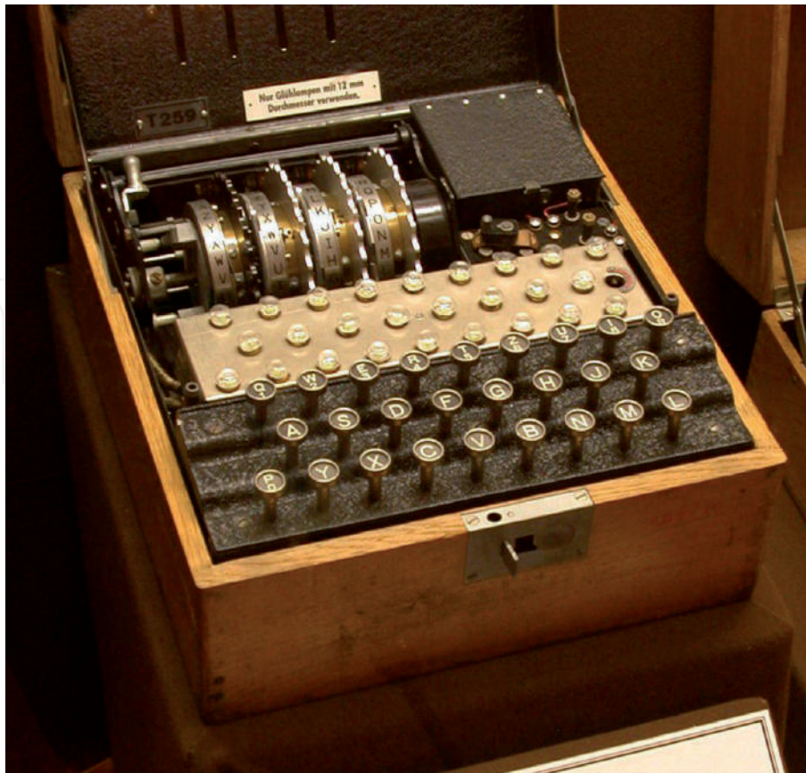
Figure 1. Picture of the German Enigma machine which was used to code military communications. Taken from Wikimedia Commons.
