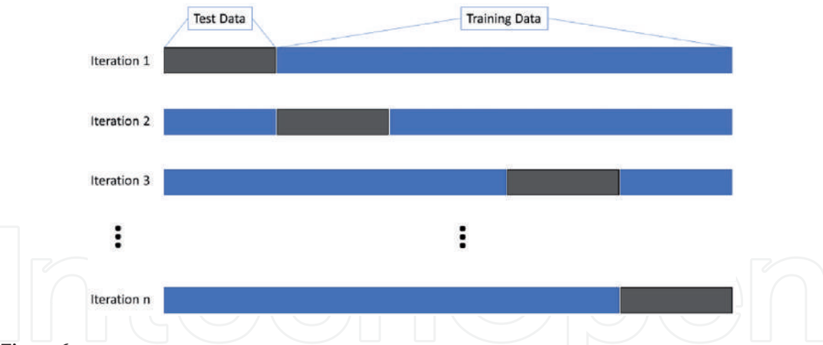
Figure 6. Example of a set of cross validation splits. There are n splits for the number of iterations desired and the results of all iterations are averaged to assess the generalized performance of a model trained on a dataset.
