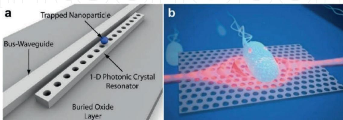
**Figure 7.** Photonic crystal optical tweezers. (a) Schematic representation of a single-dimensional photonic crystal resonator capturing a single nanoparticle [24]. (b) Schematic representation of a two-dimensional photonic crystal resonator capturing a single *E. coli* [25].
