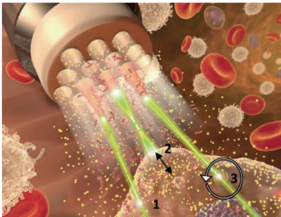
**Figure 5.** This schematic shows a versatile fiber-based optical tweezers: number 1 indicates the capture, transport, and sorting of cells, number 2 indicates the optical stretching and deformation of cells, and numbers 3 indicates the optical rotation of cells.
