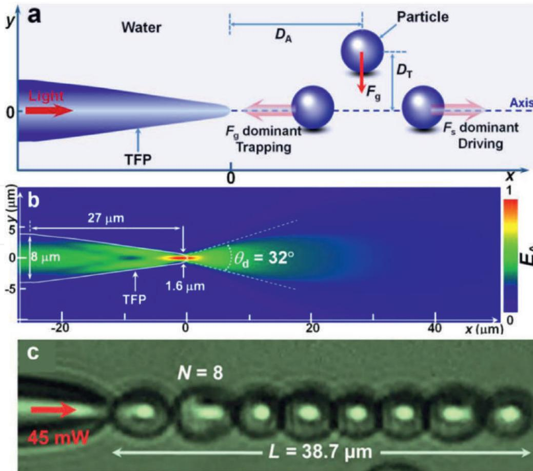
**Figure 4.** The basic principle of the fiber-based optical tweezers. (a) Schematic diagram of the optical gradient force ( $F_g$ ) and scattering force ( $F_s$ ) applied to the microparticles by the fiber-based optical tweezers. (b) Simulation of electric field intensity distribution of the fiber-based optical tweezers. (c) A chain of yeast cells was trapped by the fiber-based optical tweezers [17].
