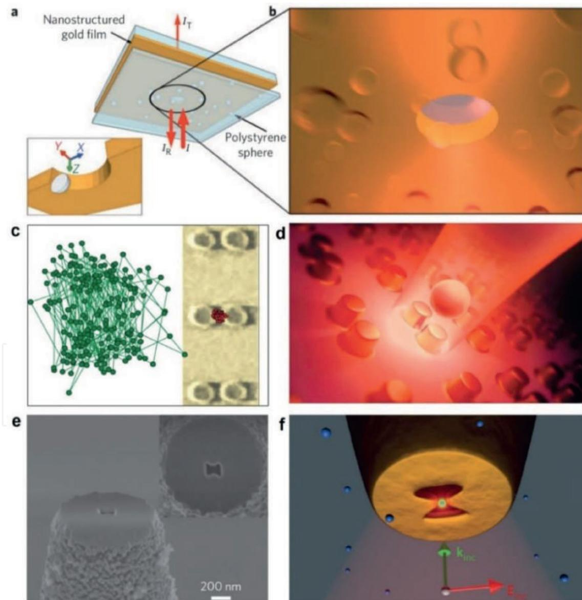
**Figure 8.** Plasmon optical tweezers. (a) Schematic diagram of a metal film having nanopores. (b) Schematic diagram of magnified metal nanopore capture nanoparticles. (c) SEM image of the metal nano-antenna structure and motion trajectory after the nanoparticles are captured. (d) Schematic representation of metal nano-antenna structures [28]. (e) SEM image of a metal nano-bowtie structure. (f) Schematic diagram of metal bow nanostructure [29].
