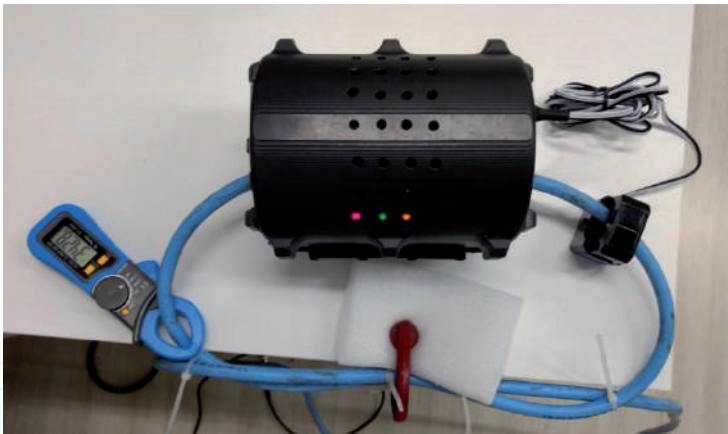
Figure 15. Device operating in a test setup with 34 a current.
