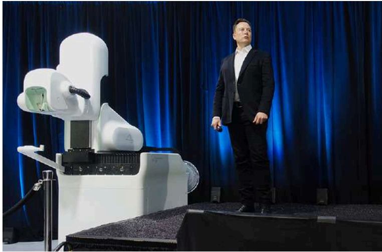
FIGURE 10.5 Elon Musk stands next to a machine for inserting a Neuralink implant in the human brain. This implant is designed to make it possible for people to operate devices like smartphones and computers using their minds. (credit: “Elon Musk and the Neuralink Future” by Steve Jurvetson/Flickr, CC BY 2.0)
