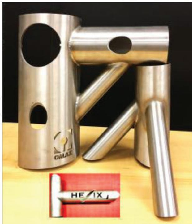
**Figure 14.** AWJ-cut “Fish mouth” weld joints.
