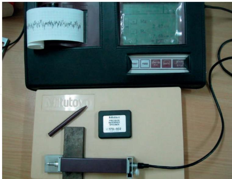
Figure 7. Measurement of surface roughness.
