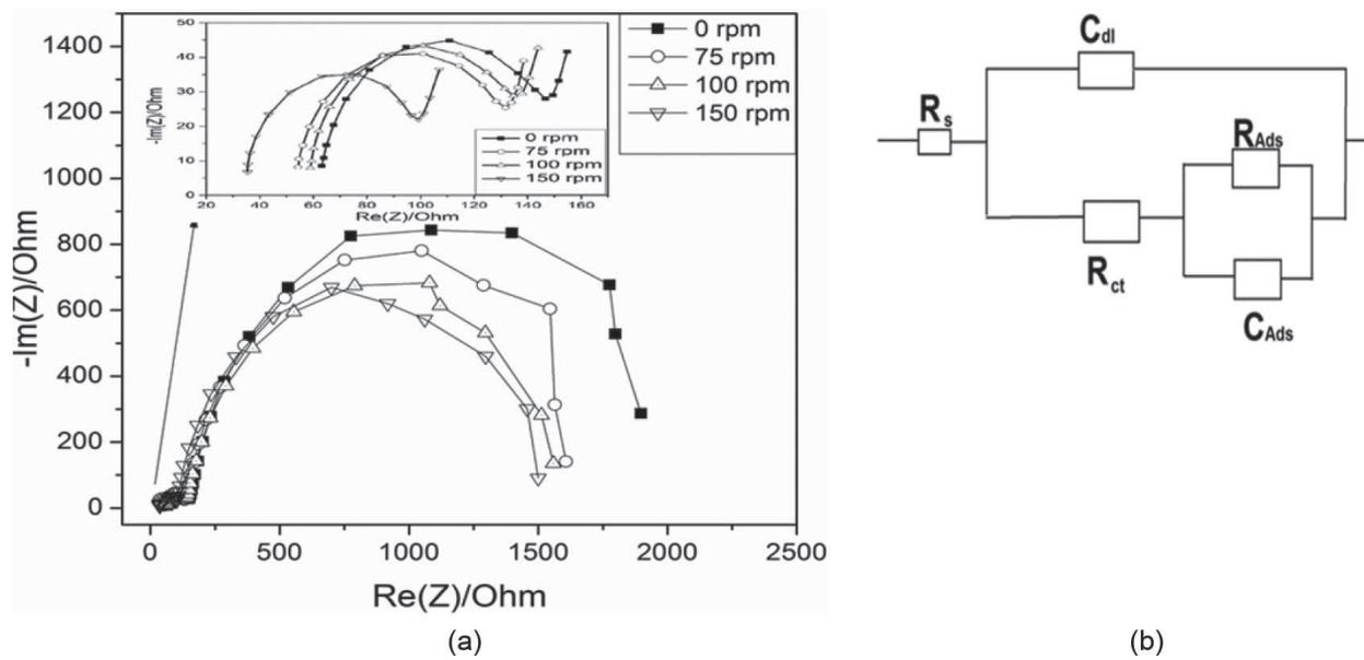
**Figure 3.** (a) Nyquist plots of the Al anode in an aqueous textile wastewater solution at 25°C temperature and varying electrode speed of rotation. (b) Equivalent circuits utilized to fit the Nyquist plots.
