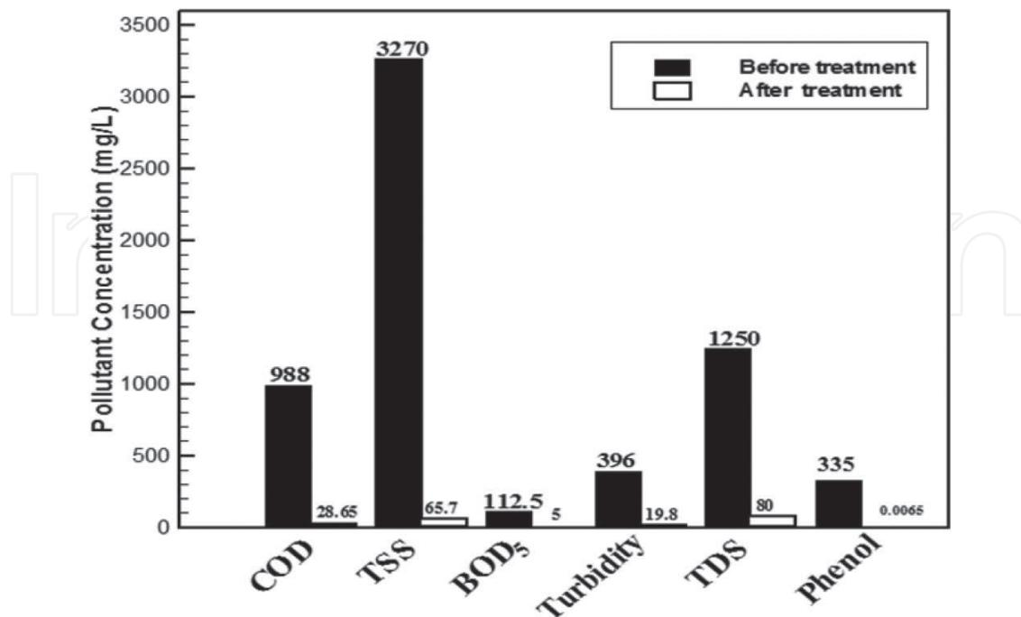
**Figure 2.** The removal efficacy of several parameters of the textile wastewater using the best operating condition.
