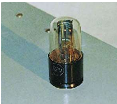
Figure 21.5 The photoelectric effect can be observed by allowing light to fall on the metal plate in this evacuated tube. Electrons ejected by the light are collected on the collector wire and measured as a current. A retarding voltage between the collector wire and plate can then be adjusted so as to determine the energy of the ejected electrons. (credit: P. P. Urone)
