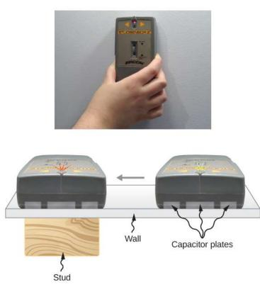
Figure 8.18 An electronic stud finder is used to detect wooden studs behind drywall. (credit top: modification of work by Jane Whitney)
