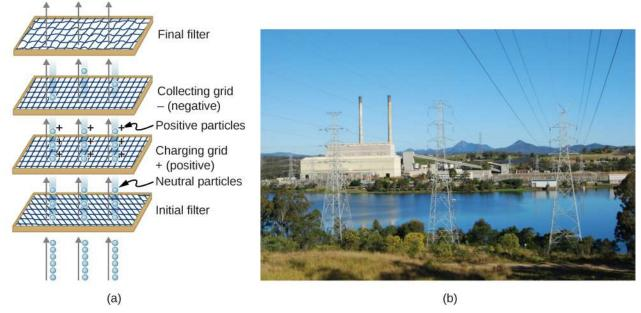
**Figure 7.45** (a) Schematic of an electrostatic precipitator. Air is passed through grids of opposite charge. The first grid charges airborne particles, while the second attracts and collects them. (b) The dramatic effect of electrostatic precipitators is seen by the absence of smoke from this power plant. (credit b: modification of work by "Cmdalgleish"/Wikimedia Commons)
