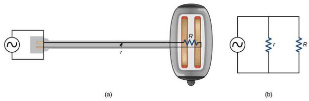
Figure 10.41 A short circuit is an undesired low-resistance path across a voltage source. (a) Worn insulation on the wires of a toaster allow them to come into contact with a low resistance *r*. Since  $P = V^2/r$ , thermal power is created so rapidly that the cord melts or burns. (b) A schematic of the short circuit.
