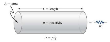
**Figure 9.15** A model of a resistor as a uniform cylinder of length *L* and cross-sectional area *A*. Its resistance to the flow of current is analogous to the resistance posed by a pipe to fluid flow. The longer the cylinder, the greater its resistance. The larger its cross-sectional area *A*, the smaller its resistance.
