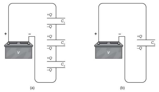
**Figure 8.11** (a) Three capacitors are connected in series. The magnitude of the charge on each plate is *Q*. (b) The network of capacitors in (a) is equivalent to one capacitor that has a smaller capacitance than any of the individual capacitances in (a), and the charge on its plates is *Q*.
