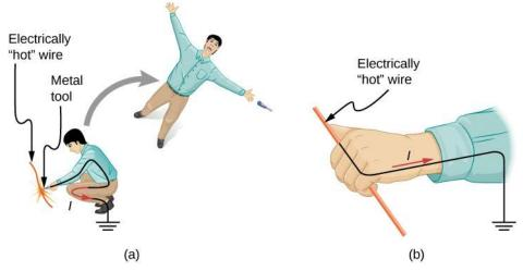
**Figure 10.42** An electric current can cause muscular contractions with varying effects. (a) The victim is "thrown" backward by involuntary muscle contractions that extend the legs and torso. (b) The victim can't let go of the wire that is stimulating all the muscles in the hand. Those that close the fingers are stronger than those that open them.
