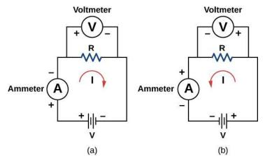
**Figure 9.19** The experimental set-up used to determine if a resistor is an ohmic or nonohmic device. (a) When the battery is attached, the current flows in the clockwise direction and the voltmeter and ammeter have positive readings. (b) When the leads of the battery are switched, the current flows in the counterclockwise direction and the voltmeter and ammeter have negative readings.
