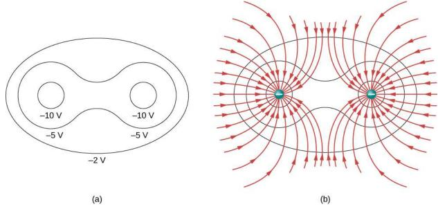
**Figure 7.32** (a) These equipotential lines might be measured with a voltmeter in a laboratory experiment. (b) The corresponding electric field lines are found by drawing them perpendicular to the equipotentials. Note that these fields are consistent with two equal negative charges. For a three-dimensional version, play with the first media link.
