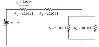
Figure 10.18 To find the unknown voltage, we must first find the equivalent resistance of the circuit.
