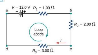
**Figure 10.21** A simple loop with no junctions. Kirchhoff's loop rule states that the algebraic sum of the voltage differences is equal to zero.
