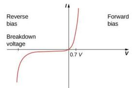
**Figure 9.22** When the voltage across the diode is negative and small, there is very little current flow through the diode. As the voltage reaches the breakdown voltage, the diode conducts. When the voltage across the diode is positive and greater than 0.7 V (the actual voltage value depends on the diode), the diode conducts. As the voltage applied increases, the current through the diode increases, but the voltage across the diode remains approximately 0.7 V.
