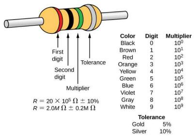
**Figure 9.16** Many resistors resemble the figure shown above. The four bands are used to identify the resistor. The first two colored bands represent the first two digits of the resistance of the resistor. The third color is the multiplier. The fourth color represents the tolerance of
