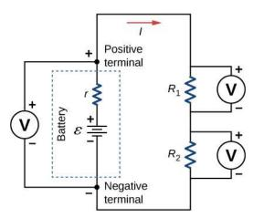
**Figure 10.36** To measure potential differences in this series circuit, the voltmeter (V) is placed in parallel with the voltage source or either of the resistors. Note that terminal voltage is measured between the positive terminal and the negative terminal of the battery or voltage source. It is not possible to connect a voltmeter directly across the emf without including the internal resistance *r* of the battery.
