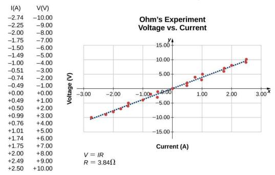
Figure 9.20 A resistor is placed in a circuit with a battery. The voltage applied varies from -10.00 V to +10.00 V, increased by 1.00-V
