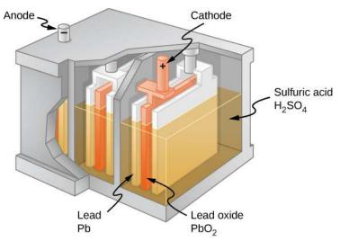
**Figure 10.4** Chemical reactions in a lead-acid cell separate charge, sending negative charge to the anode, which is connected to the lead plates. The lead oxide plates are connected to the positive or cathode terminal of the cell. Sulfuric acid conducts the charge, as well as participates in the chemical reaction.
