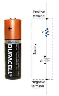
**Figure 10.6** A battery can be modeled as an idealized emf ( $\epsilon$ ) with an internal resistance (r). The terminal voltage of the battery is  $V_{\text{terminal}} = \epsilon - Ir$ .
