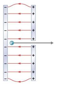
**Figure 7.46** Parallel conducting plates with opposite charges on them create a relatively uniform electric field used to accelerate electrons to the right. Those that go through the hole can be used to make a TV or computer screen glow or to produce X- rays.
