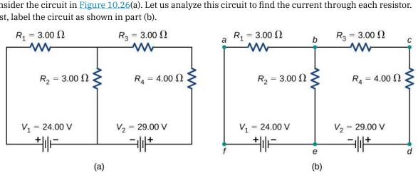
Figure 10.26 (a) A multi-loop circuit. (b) Label the circuit to help with orientation.
