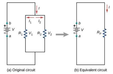
**Figure 10.14** (a) Two resistors connected in parallel to a voltage source. (b) The original circuit is reduced to an equivalent resistance and a voltage source.
