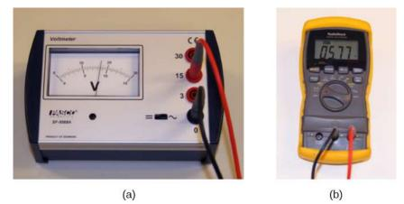
Figure 10.37 (a) An analog voltmeter uses a galvanometer to measure the voltage. (b) Digital meters use an analog-to-digital converter to measure the voltage. (credit: modification of works by Joseph J. Trout)
