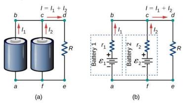
**Figure 10.33** (a) Two batteries connect in parallel to a load resistor. (b) The circuit diagram shows the shows battery as an emf source and an internal resistor. The two emf sources have identical emfs (each labeled by  $\varepsilon$ ) connected in parallel that produce the same emf.
