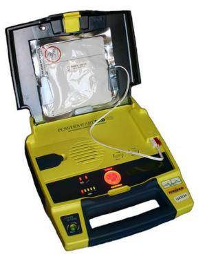
**Figure 8.16** Automated external defibrillators are found in many public places. These portable units provide verbal instructions for use in the important first few minutes for a person suffering a cardiac attack. (credit: Owain Davies)
