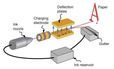
**Figure 7.44** The nozzle of an ink-jet printer produces small ink droplets, which are sprayed with electrostatic charge. Various computerdriven devices are then used to direct the droplets to the correct positions on a page.
