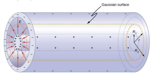
**Figure 8.7** A cylindrical capacitor consists of two concentric, conducting cylinders. Here, the charge on the outer surface of the inner cylinder is positive (indicated by +) and the charge on the inner surface of the outer cylinder is negative (indicated by -).
