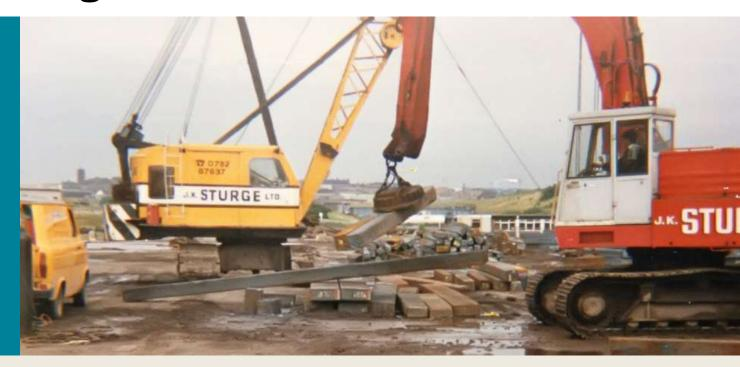
**Figure 11.1** An industrial electromagnet is capable of lifting thousands of pounds of metallic waste. (credit: modification of work by "BedfordAl"/Flickr)
