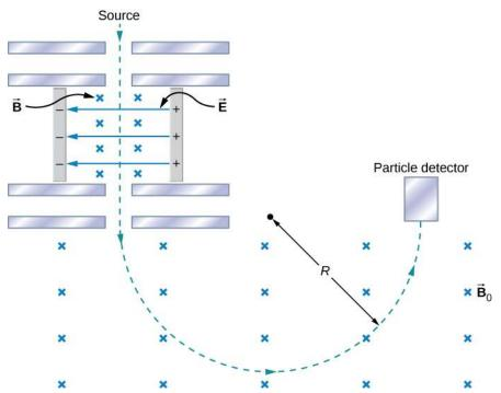
**Figure 11.19** A schematic of the Bainbridge mass spectrometer, showing charged particles leaving a source, followed by a velocity selector where the electric and magnetic forces are balanced, followed by a region of uniform magnetic field where the particle is ultimately detected.
