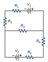
**Figure 10.19** This circuit cannot be reduced to a combination of series and parallel connections. However, we can use Kirchhoff's rules to analyze it.
