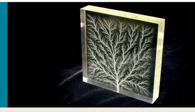
**Figure 8.1** The tree-like branch patterns in this clear Plexiglas® block are known as a Lichtenberg figure, named for the German physicist Georg Christof Lichtenberg (1742–1799), who was the first to study these patterns. The "branches" are created by the dielectric breakdown produced by a strong electric field. (credit: modification of work by Bert Hickman)
