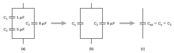
**Figure 8.13** (a) This circuit contains both series and parallel connections of capacitors. (b)  $C_1$  and  $C_2$  are in series; their equivalent capacitance is  $C_S$ . (c) The equivalent capacitance  $C_S$  is connected in parallel with  $C_3$ . Thus, the equivalent capacitance of the entire network is the sum of  $C_S$  and  $C_3$ .
