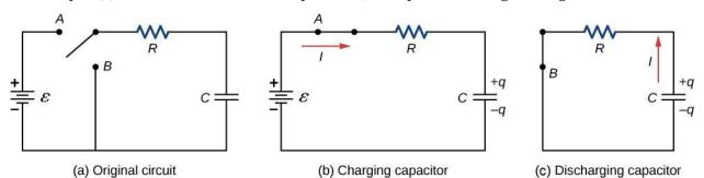
**Figure 10.38** (a) An *RC* circuit with a two-pole switch that can be used to charge and discharge a capacitor. (b) When the switch is moved to position *A*, the circuit reduces to a simple series connection of the voltage source, the resistor, the capacitor, and the switch. (c) When the switch is moved to position *B*, the circuit reduces to a simple series connection of the resistor, the capacitor, and the switch. The voltage source is removed from the circuit.
