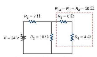
(b) Step 1: resistors  $R_3$  and  $R_4$  in series
