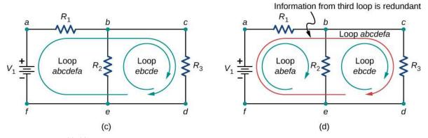
Figure 10.25 Panels (a)–(c) are sufficient for the analysis of the circuit. In each case, the two loops shown contain all the circuit elements necessary to solve the circuit completely. Panel (d) shows three loops used, which is more than necessary. Any two loops in the system will contain all information needed to solve the circuit. Adding the third loop provides redundant information.
