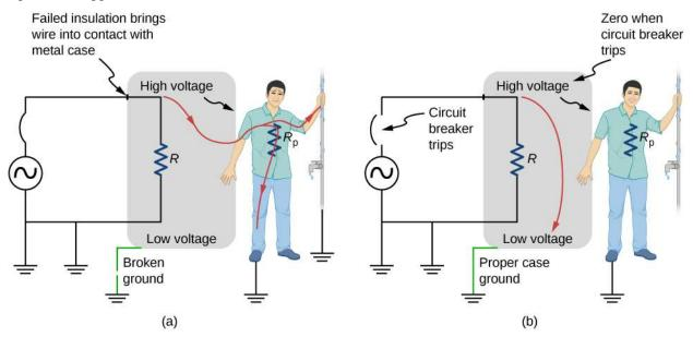
**Figure 10.45** Worn insulation allows the live/hot wire to come into direct contact with the metal case of this appliance. (a) The ground connection being broken, the person is severely shocked. The appliance may operate normally in this situation. (b) With a proper ground, the circuit breaker trips, forcing repair of the appliance.
