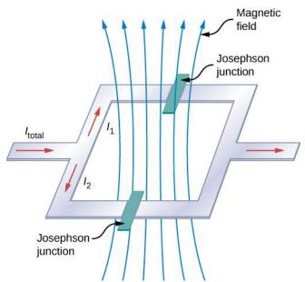
**Figure 9.29** The SQUID (superconducting quantum interference device) uses a superconducting current loop and two Josephson junctions to detect magnetic fields as low as  $10^{-14}$  T (Earth's magnet field is on the order of  $0.3 \times 10^{-5}$  T).
