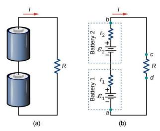
**Figure 10.31** (a) Two batteries connected in series with a load resistor. (b) The circuit diagram of the two batteries and the load resistor, with each battery modeled as an idealized emf source and an internal resistance.
