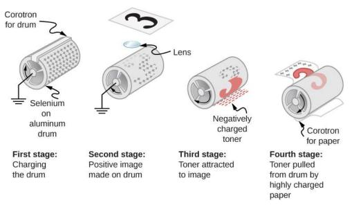
**Figure 7.42** Xerography is a dry copying process based on electrostatics. The major steps in the process are the charging of the photoconducting drum, transfer of an image, creating a positive charge duplicate, attraction of toner to the charged parts of the drum, and transfer of toner to the paper. Not shown are heat treatment of the paper and cleansing of the drum for the next copy.
