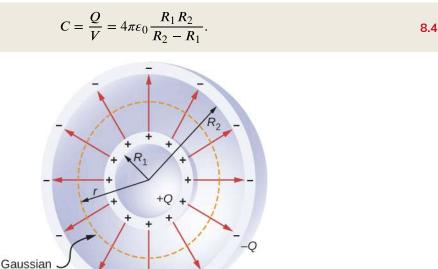
Figure 8.6 A spherical capacitor consists of two concentric conducting spheres. Note that the charges on a conductor reside on its surface.
