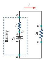
**Figure 10.7** Schematic of a voltage source and its load resistor *R*. Since the internal resistance *r* is in series with the load, it can significantly affect the terminal voltage and the current delivered to the load.
