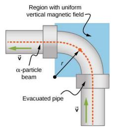
Figure 11.10 Top view of the beam deflector setup.
