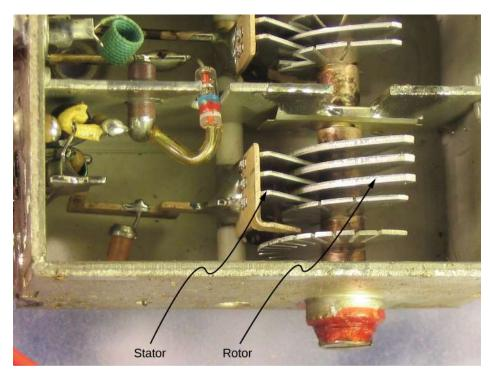
**Figure 8.8** In a variable air capacitor, capacitance can be tuned by changing the effective area of the plates. (credit: modification of work by Robbie Sproule)
