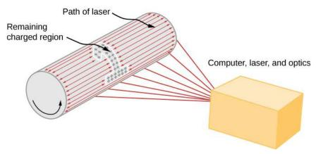
**Figure 7.43** In a laser printer, a laser beam is scanned across a photoconducting drum, leaving a positively charged image. The other steps for charging the drum and transferring the image to paper are the same as in xerography. Laser light can be very precisely controlled, enabling laser printers to produce high-quality images.
