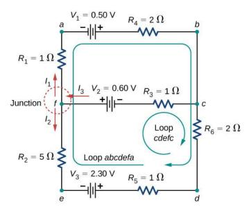
**Figure 10.29** This circuit is combination of series and parallel configurations of resistors and voltage sources. This circuit cannot be analyzed using the techniques discussed in <u>Electromotive Force</u> but can be analyzed using Kirchhoff's rules.
