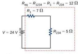
(d) Step 3: resistors  $R_1$  and  $R_{234}$  in series
