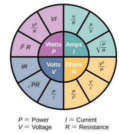
Figure 9.26 This circle shows a summary of the equations for the relationships between power, current, voltage, and resistance.
