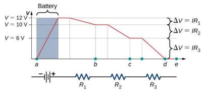
**Figure 10.22** A voltage graph as we travel around the circuit. The voltage increases as we cross the battery and decreases as we cross each resistor. Since the resistance of the wire is quite small, we assume that the voltage remains constant as we cross the wires connecting the components.
