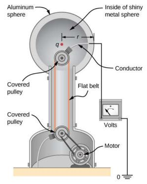
**Figure 7.18** The voltage of this demonstration Van de Graaff generator is measured between the charged sphere and ground. Earth's potential is taken to be zero as a reference. The potential of the charged conducting sphere is the same as that of an equal point charge at its center.
