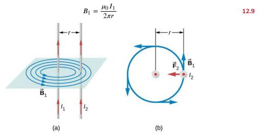
**Figure 12.9** (a) The magnetic field produced by a long straight conductor is perpendicular to a parallel conductor, as indicated by righthand rule (RHR)-2. (b) A view from above of the two wires shown in (a), with one magnetic field line shown for wire 1. RHR-1 shows that the force between the parallel conductors is attractive when the currents are in the same direction. A similar analysis shows that the force is repulsive between currents in opposite directions.
