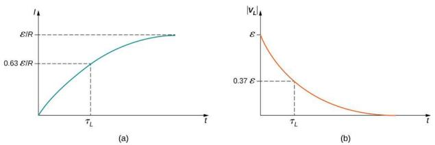
**Figure 14.13** Time variation of (a) the electric current and (b) the magnitude of the induced voltage across the coil in the circuit of <u>Figure</u> <u>14.12</u>(b).
