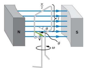
**Figure 13.28** A generator with a single rectangular coil rotated at constant angular velocity in a uniform magnetic field produces an emf that varies sinusoidally in time. Note the generator is similar to a motor, except the shaft is rotated to produce a current rather than the other way around.
