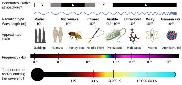
Figure 16.17 The electromagnetic spectrum, showing the major categories of electromagnetic waves.
