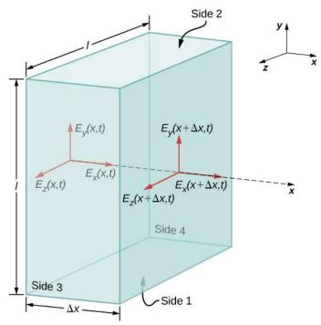
**Figure 16.6** The surface of a rectangular box of dimensions  $l \times l \times \Delta x$  is our Gaussian surface. The electric field shown is from an electromagnetic wave propagating along the *x*-axis.
