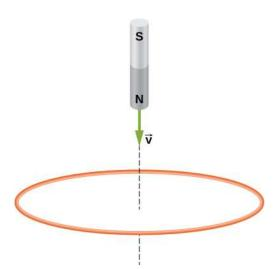
**13.** The accompanying figure shows a conducting ring at various positions as it moves through a magnetic field. What is the sense of the induced emf for each of those positions?
