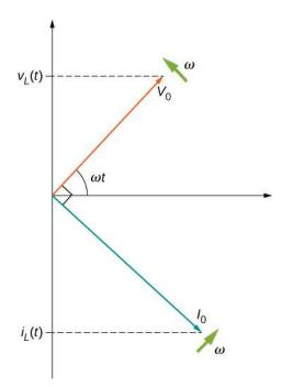
**Figure 15.10** The phasor diagram for the inductor of <u>Figure 15.9</u>. The current phasor lags the voltage phasor by  $\pi/2$  rad as they both rotate with the same angular frequency.
