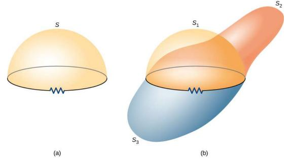
**Figure 13.5** (a) A circuit bounding an arbitrary open surface *S*. The planar area bounded by the circuit is not part of *S*. (b) Three arbitrary open surfaces bounded by the same circuit. The value of  $\Phi_m$  is the same for all these surfaces.
