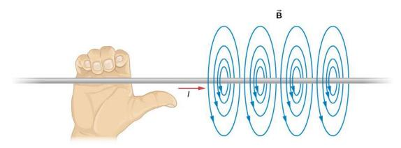
Figure 12.6 Some magnetic field lines of an infinite wire. The direction of **B** can be found with a form of the right-hand rule.
