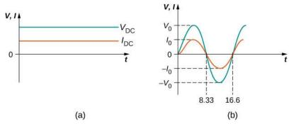
**Figure 15.2** (a) The dc voltage and current are constant in time, once the current is established. (b) The voltage and current versus time are quite different for ac power. In this example, which shows 60-Hz ac power and time *t* in milliseconds, voltage and current are sinusoidal and are in phase for a simple resistance circuit. The frequencies and peak voltages of ac sources differ greatly.
