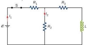
**60.** For the circuit shown below, find the current through the inductor  $2.0 \times 10^{-5}$  s after the switch is reopened.
