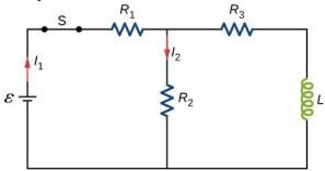
**61**. Show that for the circuit shown below, the initial energy stored in the inductor,  $LI^2(0)/2$ , is equal to the total energy eventually dissipated in the resistor,
