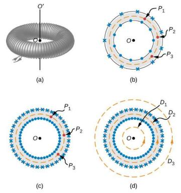
Figure 12.22 (a) A toroid is a coil wound into a donut-shaped object. (b) A loosely wound toroid does not have cylindrical symmetry. (c) In a tightly wound toroid, cylindrical symmetry is a very good approximation. (d) Several paths of integration for Ampère's law.
