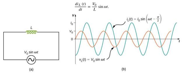
Figure 15.9 (a) An inductor connected across an ac generator. (b) The current  $i_L(t)$  through the inductor and the voltage  $v_L(t)$  across the inductor. Here  $i_L(t)$  lags  $v_L(t)$  by  $\pi/2$  rad.
