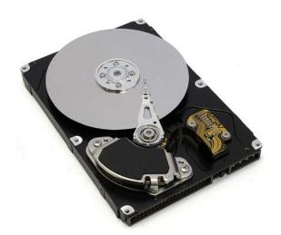
**Figure 12.28** The inside of a hard disk drive. The silver disk contains the information, whereas the thin stylus on top of the disk reads and writes information to the disk.
