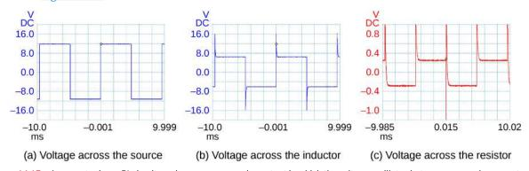
**Figure 14.15** A generator in an *RL* circuit produces a square-pulse output in which the voltage oscillates between zero and some set value. These oscilloscope traces show (a) the voltage across the source; (b) the voltage across the inductor; (c) the voltage across the resistor.
