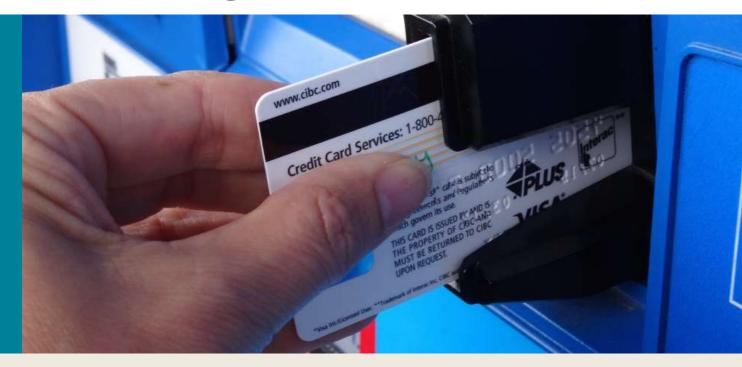
**Figure 13.1** The black strip found on the back of credit cards and driver's licenses is a very thin layer of magnetic material with information stored on it. Reading and writing the information on the credit card is done with a swiping motion. The physical reason why this is necessary is called electromagnetic induction and is discussed in this chapter. (credit: modification of work by Jane Whitney)
