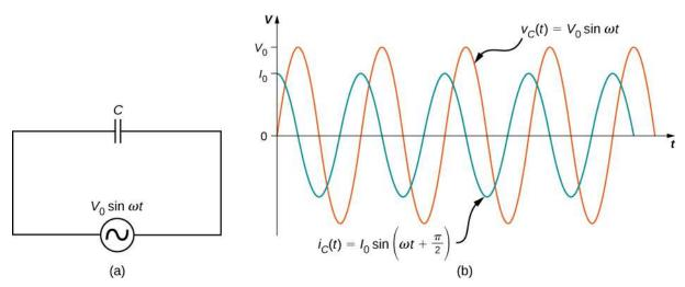
**Figure 15.7** (a) A capacitor connected across an ac generator. (b) The current  $i_C(t)$  through the capacitor and the voltage  $v_C(t)$  across the capacitor. Notice that  $i_C(t)$  leads  $v_C(t)$  by  $\pi/2$  rad.
