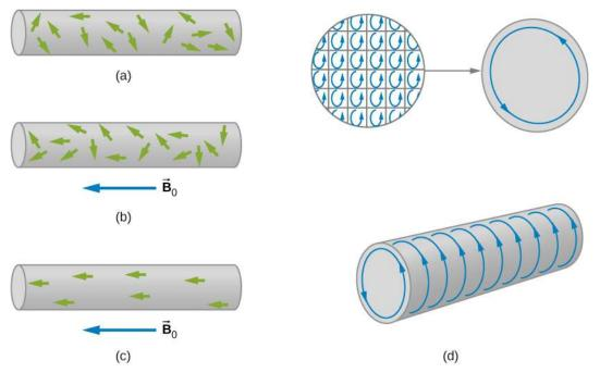
**Figure 12.23** The alignment process in a paramagnetic material filling a solenoid (not shown). (a) Without an applied field, the magnetic dipoles are randomly oriented. (b) With a field, partial alignment occurs. (c) An equivalent representation of part (b). (d) The internal currents cancel, leaving an effective surface current that produces a magnetic field similar to that of a finite solenoid.
