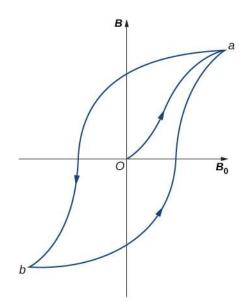
**Figure 12.26** A typical hysteresis loop for a ferromagnet. When the material is first magnetized, it follows a curve from 0 to *a*. When  $B_0$  is reversed, it takes the path shown from *a* to *b*. If  $B_0$  is reversed again, the material follows the curve from *b* to *a*.
