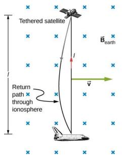
**Figure 13.15** Motional emf as electrical power conversion for the space shuttle was the motivation for the tethered satellite experiment. A 5-kV emf was predicted to be induced in the 20-km tether while moving at orbital speed in Earth's magnetic field. The circuit is completed by a return path through the stationary ionosphere.
