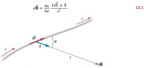
**Figure 12.2** A current element  $Id\vec{l}$  produces a magnetic field at point *P* given by the Biot-Savart law.
