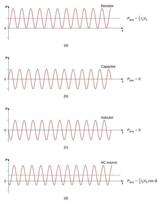
Figure 15.16 Graph of instantaneous power for various circuit elements. (a) For the resistor,  $P_{ave} = I_0 V_0/2$ , whereas for (b) the capacitor and (c) the inductor,  $P_{ave} = 0$ . (d) For the source,  $P_{ave} = I_0 V_0 (\cos \phi)/2$ , which may be positive, negative, or zero, depending on  $\phi$ .
