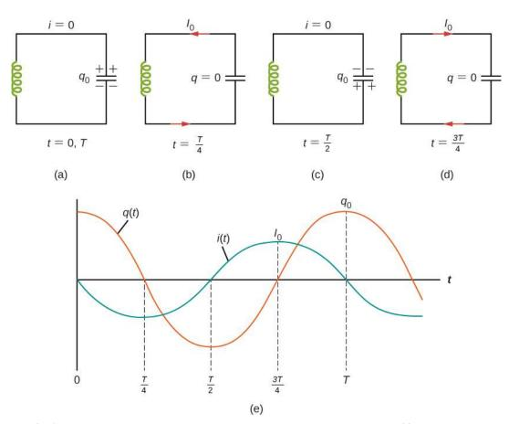
**Figure 14.16** (a–d) The oscillation of charge storage with changing directions of current in an *LC* circuit. (e) The graphs show the distribution of charge and current between the capacitor and inductor.
