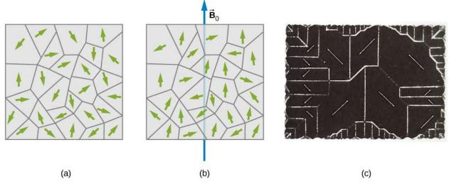
**Figure 12.24** (a) Domains are randomly oriented in an unmagnetized ferromagnetic sample such as iron. The arrows represent the orientations of the magnetic dipoles within the domains. (b) In an applied magnetic field, the domains align somewhat with the field. (c) The domains of a single crystal of nickel. The white lines show the boundaries of the domains. These lines are produced by iron oxide powder sprinkled on the crystal.
