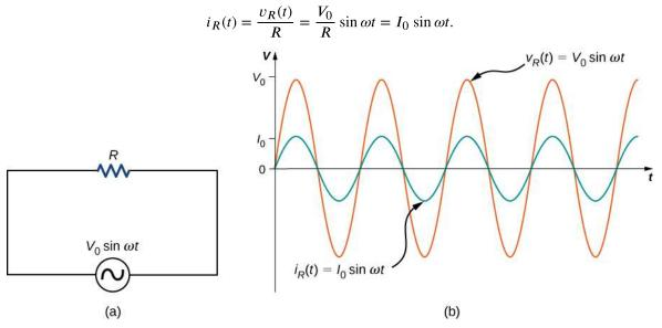
**Figure 15.5** (a) A resistor connected across an ac voltage source. (b) The current  $i_R(t)$  through the resistor and the voltage  $v_R(t)$  across the resistor. The two quantities are in phase.
