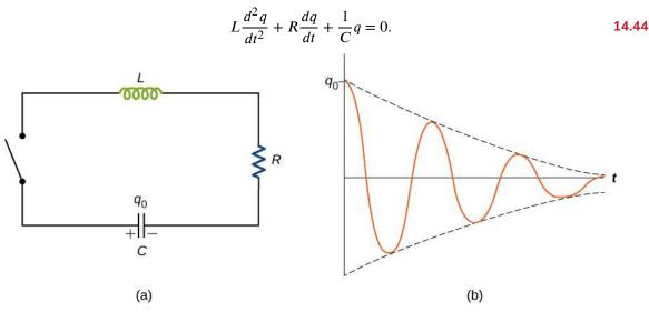
Figure 14.17 (a) An *RLC* circuit. Electromagnetic oscillations begin when the switch is closed. The capacitor is fully charged initially. (b) Damped oscillations of the capacitor charge are shown in this curve of charge versus time, or q versus t. The capacitor contains a charge  $q_0$  before the switch is closed.
