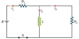
**59**. For the circuit shown below,  $\varepsilon = 50$  V,  $R_1 = 10 \Omega_{,,}$  $R_2 = R_3 = 19.4 \Omega_{,,}$  and L = 2.0 mH. Find the values of  $I_1$  and  $I_2$  (a) immediately after switch S is closed, (b) a long time after S is closed, (c) immediately after S is reopened, and (d) a long time after S is reopened.
