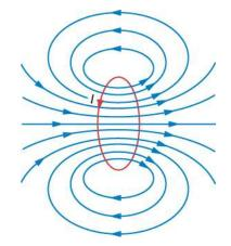
Figure 12.12 Sketch of the magnetic field lines of a circular current loop.
