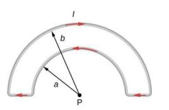
**19**. The accompanying figure shows a current loop consisting of two concentric circular arcs and two perpendicular radial lines. Determine the magnetic field at point P.
