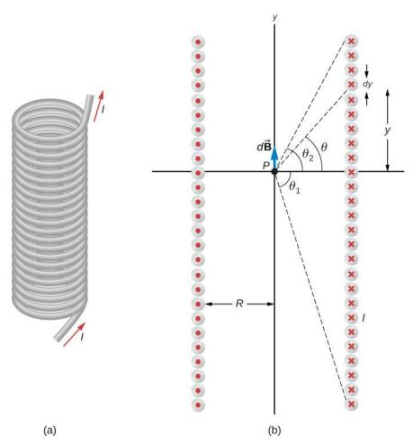
**Figure 12.19** (a) A solenoid is a long wire wound in the shape of a helix. (b) The magnetic field at the point *P* on the axis of the solenoid is the net field due to all of the current loops.
