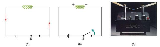
**Figure 13.8** (a) A solenoid connected to a source of emf. (b) Opening switch S terminates the current, which in turn induces an emf in the solenoid. (c) A potential difference between the ends of the sharply pointed rods is produced by inducing an emf in a coil. This potential difference is large enough to produce an arc between the sharp points.
