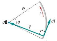
Figure 12.4 A wire segment carrying a current *I*. The path  $d\vec{l}$  and radial direction  $\hat{\mathbf{r}}$  are indicated.
