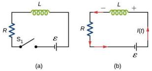
**57**. The current in the *RL* circuit shown below reaches half its maximum value in 1.75 ms after the switch  $S_1$  is thrown. Determine (a) the time constant of the circuit and (b) the resistance of
