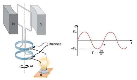
**Figure 13.29** The emf of a generator is sent to a light bulb with the system of rings and brushes shown. The graph gives the emf of the generator as a function of time, where  $\epsilon_0$  is the peak emf. The period is  $T = 1/f = 2\pi/\omega$ , where *f* is the frequency.
