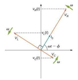
Figure 15.12 The phasor diagram for the *RLC* series circuit of Figure 15.11.
