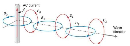
Figure 16.4 How changing  $\vec{E}$  and  $\vec{B}$  fields propagate through space.
