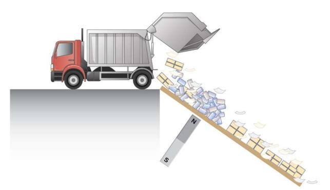
**Figure 13.24** Metals can be separated from other trash by magnetic drag. Eddy currents and magnetic drag are created in the metals sent down this ramp by the powerful magnet beneath it. Nonmetals move on.
