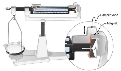
**Figure 13.23** Magnetic damping of this sensitive balance slows its oscillations. Since Faraday's law of induction gives the greatest effect for the most rapid change, damping is greatest for large oscillations and goes to zero as the motion stops.
