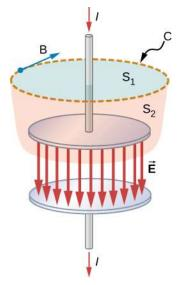
**Figure 16.3** The currents through surface  $S_1$  and surface  $S_2$  are unequal, despite having the same boundary loop *C*.
