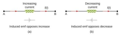
**Figure 14.8** The induced emf across an inductor always acts to oppose the change in the current. This can be visualized as an imaginary battery causing current to flow to oppose the change in (a) and reinforce the change in (b).
