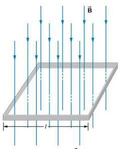
Figure 13.6 A square coil with N turns of wire with uniform magnetic field **B** directed in the downward direction, perpendicular to the coil.
