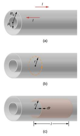
**Figure 14.11** (a) A coaxial cable is represented here by two hollow, concentric cylindrical conductors along which electric current flows in opposite directions. (b) The magnetic field between the conductors can be found by applying Ampère's law to the dashed path. (c) The cylindrical shell is used to find the magnetic energy stored in a length *l* of the cable.
