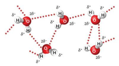
**Figure 16.19** The oscillating electric field in a microwave oven exerts a torque on water molecules because of their dipole moment, and the torque reverses direction  $4.90 \times 10^9$  times per second. Interactions between the molecules distributes the energy being pumped into them. The  $\delta^+$  and  $\delta^-$  denote the charge distribution on the molecules.
