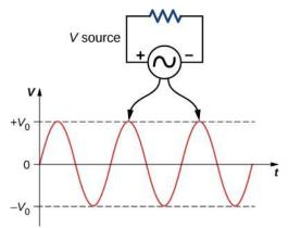
**Figure 15.3** The potential difference *V* between the terminals of an ac voltage source fluctuates, so the source and the resistor have ac sine waves on top of each other. The mathematical expression for *v* is given by  $v = V_0 \sin \omega t$ .
