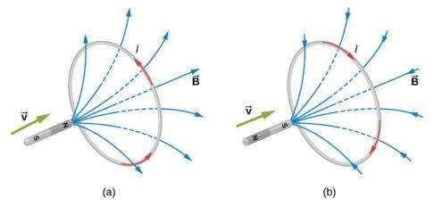
**Figure 13.7** The change in magnetic flux caused by the approaching magnet induces a current in the loop. (a) An approaching north pole induces a counterclockwise current with respect to the bar magnet. (b) An approaching south pole induces a clockwise current with respect to the bar magnet.
