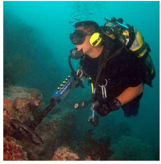
**Figure 15.19** When a metal detector comes near a piece of metal, the self-inductance of one of its coils changes. This causes a shift in the resonant frequency of a circuit containing the coil. That shift is detected by the circuitry and transmitted to the diver by means of the headphones. (credit: modification of work by Eric Lippmann, U.S. Navy)
