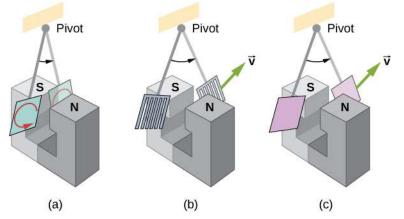
**Figure 13.20** A common physics demonstration device for exploring eddy currents and magnetic damping. (a) The motion of a metal pendulum bob swinging between the poles of a magnet is quickly damped by the action of eddy currents. (b) There is little effect on the motion of a slotted metal bob, implying that eddy currents are made less effective. (c) There is also no magnetic damping on a nonconducting bob, since the eddy currents are extremely small.
