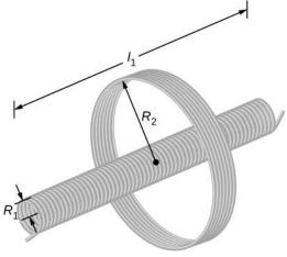
Figure 14.4 A solenoid surrounded by a coil.
