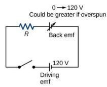
**Figure 13.32** The coil of a dc motor is represented as a resistor in this schematic. The back emf is represented as a variable emf that opposes the emf driving the motor. Back emf is zero when the motor is not turning and increases proportionally to the motor's angular velocity.
