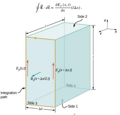
**Figure 16.7** We apply Faraday's law to the front of the rectangle by evaluating  $\oint \vec{E} \cdot d\vec{s}$  along the rectangular edge of Side 3 in the direction indicated, taking the *B* field crossing the face to be approximately its value in the middle of the area traversed.
