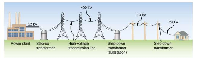
**Figure 15.20** The rms voltage from a power plant eventually needs to be stepped down from 12 kV to 240 V so that it can be safely introduced into a home. A high-voltage transmission line allows a low current to be transmitted via a substation over long distances.
