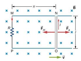
**Figure 13.12** A conducting rod is pushed to the right at constant velocity. The resulting change in the magnetic flux induces a current in the circuit.
