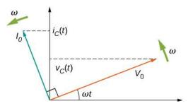
**Figure 15.8** The phasor diagram for the capacitor of <u>Figure 15.7</u>. The current phasor leads the voltage phasor by  $\pi/2$  rad as they both rotate with the same angular frequency.
