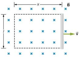
Figure 13.14 With the imaginary rectangle shown, we can use Faraday's law to calculate the induced emf in the moving rod.
