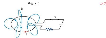
**Figure 14.5** A magnetic field is produced by the current *I* in the loop. If *I* were to vary with time, the magnetic flux through the loop would also vary and an emf would be induced in the loop.
