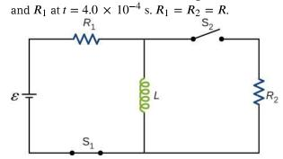
**54.** The current in the *RL* circuit shown here increases to 40% of its steady-state value in 2.0 s. What is the time constant of the circuit?
