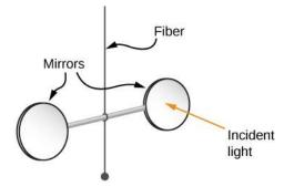
**Figure 16.14** Simplified diagram of the central part of the apparatus Nichols and Hull used to precisely measure radiation pressure and confirm Maxwell's prediction.
