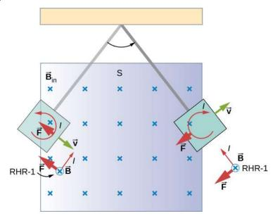
**Figure 13.21** A more detailed look at the conducting plate passing between the poles of a magnet. As it enters and leaves the field, the change in flux produces an eddy current. Magnetic force on the current loop opposes the motion. There is no current and no magnetic drag when the plate is completely inside the uniform field.
