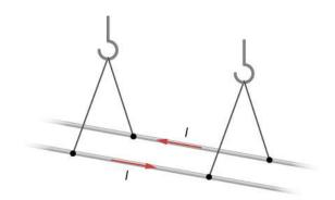
**33**. A circuit with current *I* has two long parallel wire sections that carry current in opposite directions. Find magnetic field at a point *P* near these wires that is a distance *a* from one wire and *b* from the other wire as shown in the figure.
