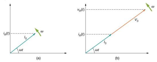
**Figure 15.6** (a) The phasor diagram representing the current through the resistor of <u>Figure 15.5</u>. (b) The phasor diagram representing both  $i_R(t)$  and  $v_R(t)$ .
