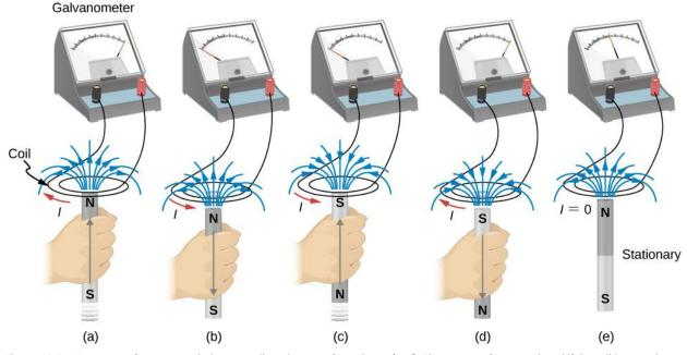
**Figure 13.2** Movement of a magnet relative to a coil produces emfs as shown (a–d). The same emfs are produced if the coil is moved relative to the magnet. This short-lived emf is only present during the motion. The greater the speed, the greater the magnitude of the emf, and the emf is zero when there is no motion, as shown in (e).
