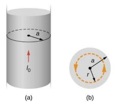
Figure 12.16 (a) A model of a current-carrying wire of radius *a* and current  $I_0$ . (b) A cross-section of the same wire showing the radius *a* and the Ampère's loop of radius *r*.
