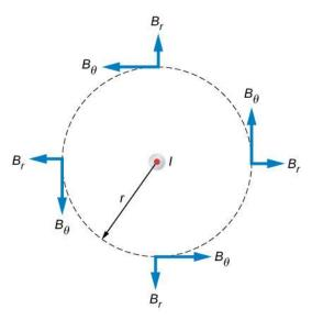
**Figure 12.15** The possible components of the magnetic field *B* due to a current *I*, which is directed out of the page. The radial component is zero because the angle between the magnetic field and the path is at a right angle.
