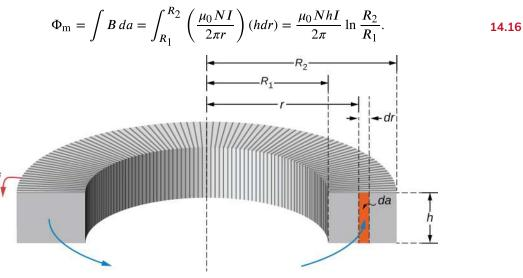
Figure 14.10 Calculating the self-inductance of a rectangular toroid.
