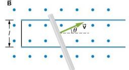
**42.** The rod shown in the accompanying figure is moving through a uniform magnetic field of strength B = 0.50 T with a constant velocity of magnitude v = 8.0 m/s. What is the potential difference between the ends of the rod? Which end of the rod is at a higher potential?
