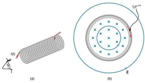
**Figure 13.18** (a) The current in a long solenoid is decreasing exponentially. (b) A cross-sectional view of the solenoid from its left end. The cross-section shown is near the middle of the solenoid. An electric field is induced both inside and outside the solenoid.
