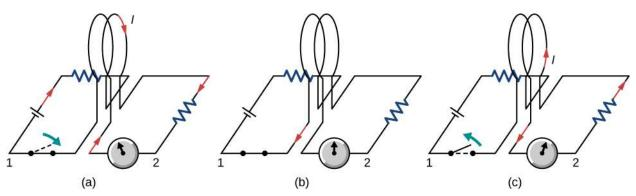
**Figure 13.3** (a) Closing the switch of circuit 1 produces a short-lived current surge in circuit 2. (b) If the switch remains closed, no current is observed in circuit 2. (c) Opening the switch again produces a short-lived current in circuit 2 but in the opposite direction from before.
