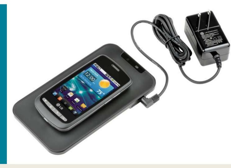
**Figure 14.1** A smartphone charging mat contains a coil that receives alternating current, or current that is constantly increasing and decreasing. The varying current induces an emf in the smartphone, which charges its battery. Note that the black box containing the electrical plug also contains a transformer (discussed in <u>Alternating-Current Circuits</u>) that modifies the current from the outlet to suit the needs of the smartphone. (credit: modification of work by "LG"/Flickr)
