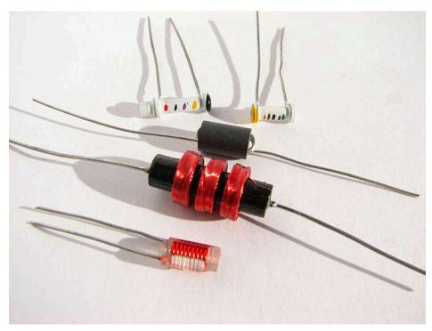
**Figure 14.7** A variety of inductors. Whether they are encapsulated like the top three shown or wound around in a coil like the bottommost one, each is simply a relatively long coil of wire. (credit: Windell Oskay)
