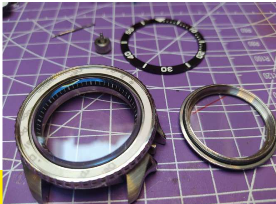
Above ♦ The dive-style watch-case with the exhibition case back and a stick-on bezel cover
