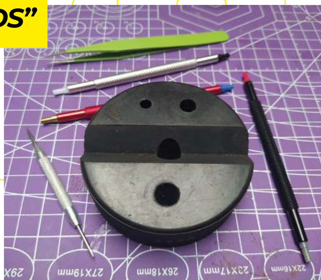
Right ♦ Some budget watchmaker’s tools; some hand setters, a dust blower, tweezers, and a bench block
