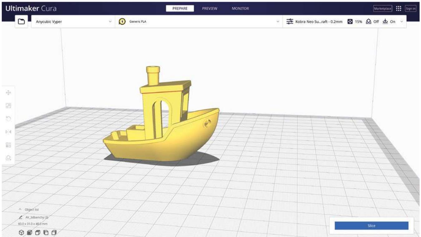
the layer height. This is the depth of each layer in the print. Smaller layers will print slower but give more detail, while thicker layers will print faster but with less detail. If you need parts to fit together, you might find that you need a thinner layer height to get the parts the exact shape needed.
