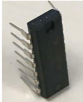
Figure 7.1: LM324 Quad OpAmp IC Pinout (Left), LM324 14-DIP package photo (Right)
