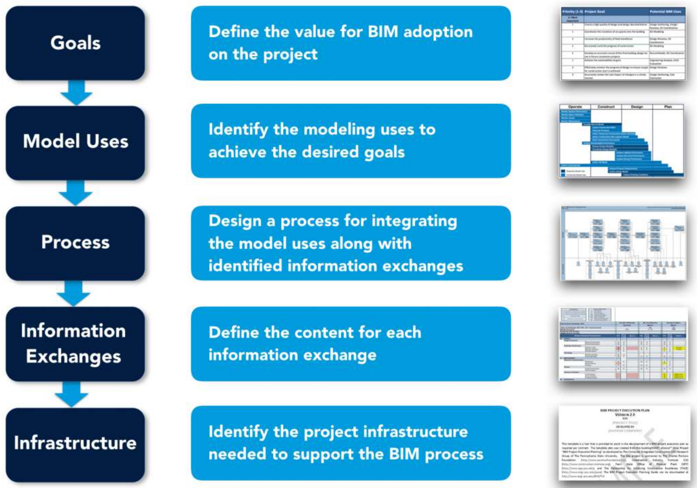
Figure i-1: BIM Project Execution Planning Procedure
