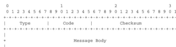
Figure 5.42: ICMP version 6 packet format
