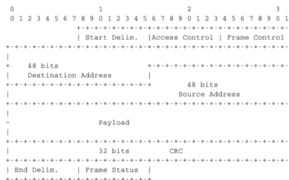
Figure 6.16: 802.5 data frame format
