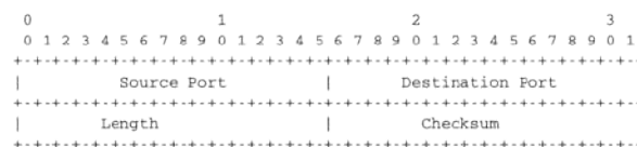
Figure 4.35: UDP Header Format
