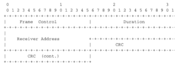
Figure 6.35: IEEE 802.11 ACK and CTS frames
