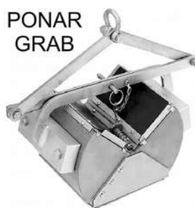
Figure 6.8: Ponar grab sampler. Source: United States Geological Survey 2004
