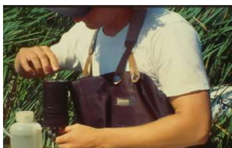
Figure 6.7: Hester dandy multiplate sampler. Source: M. Meixler
