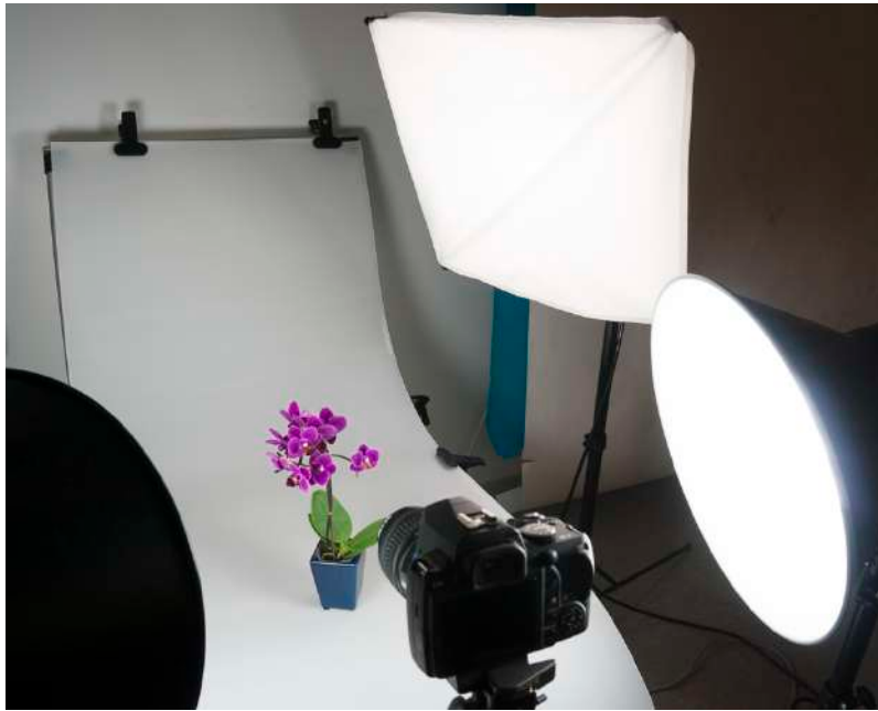
Figure 14-11. Studio lights can be equipped with various types of diffusers, including transmissive “soft boxes,” as in the photo, and reflective umbrellas.
