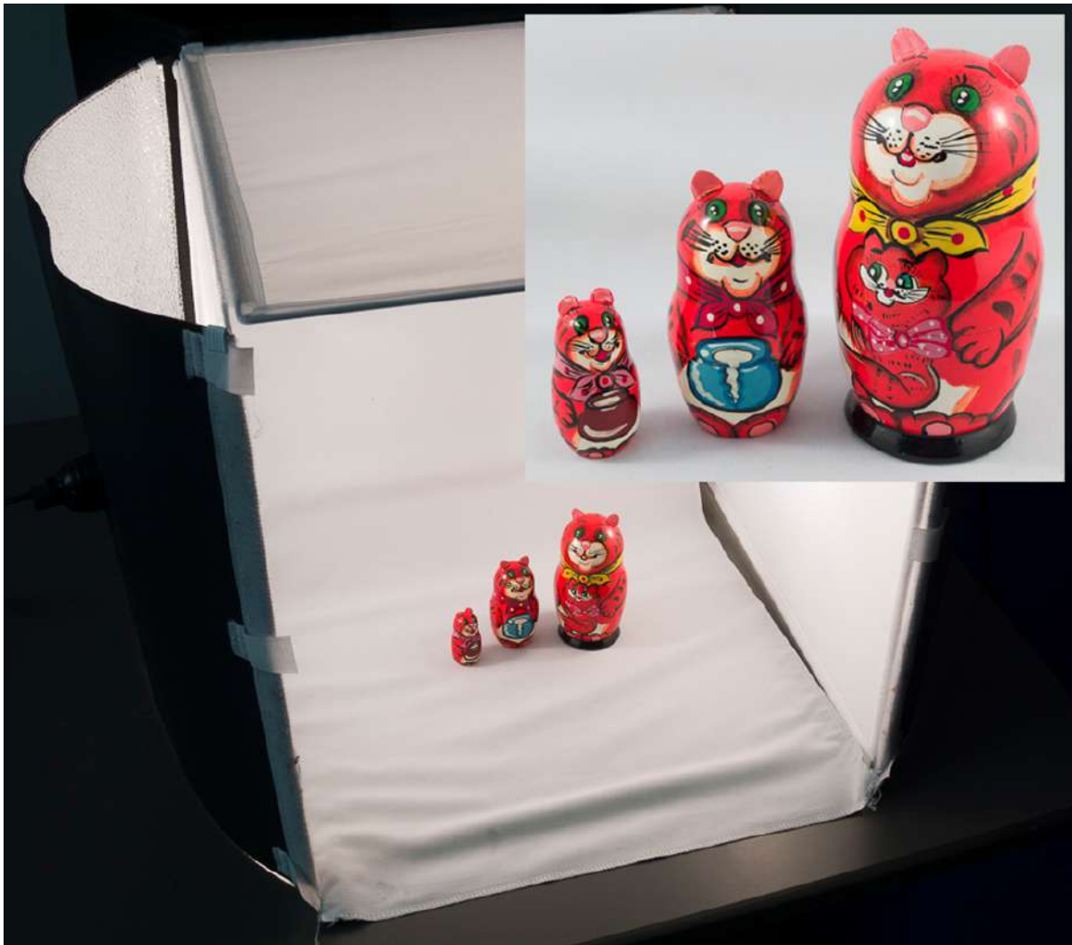
Figure 14-12. A light tent provides diffuse light for product photography.
