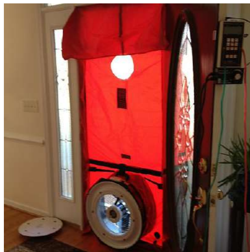
Figure 4.3: Blower door test illustration. Image description.
