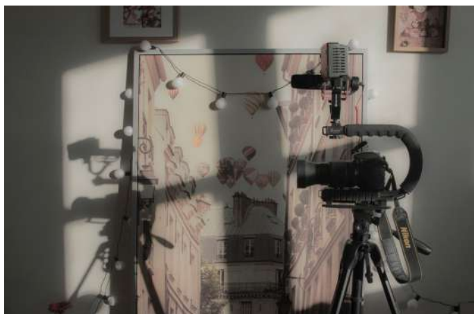
Fig. 49. A homemade rig, assembled over time from inexpensive but effective component parts. A C-grip forms the basis of it. Cold-shoe extenders allow for external accessories, including lights and microphones, to be added to the rig. This is a handheld setup that has been attached to a tripod for stationary shots without needing to be disassembled.
