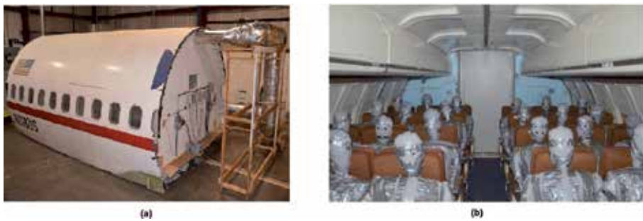
Figure 4. 5-rows B737 (a) exterior and (b) interior with inflatable heated manikins [7].
