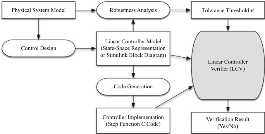
**Fig. 1.** LCV in the model-based development process.
