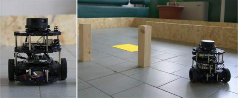
Fig. 2: The *Robotis Turtlebot 3* platform, navigating in an arena. The image on the left depicts a static robot, and the image on the right depicts the robot moving towards the destination (the yellow square), while avoiding two wooden obstacles in its route.
