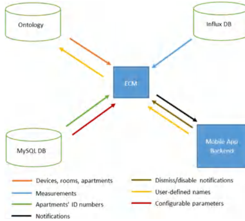
Fig. 3. Proposed architecture of a small-scale ECM system
