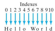
Figure 7.7: The indexing of the “Hello, World!” string.
