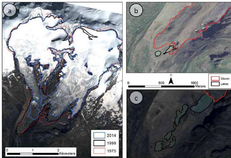
**Figure 4.** Area changes of Lys glacier and its proglacial lakes over sample years. (a) Lys glacier outlines in 1975, 1999 and 2014. Background is the orthorectified Pleiades satellite image from 2014. (b) the glacier terminus and two proglacial lakes in 2006. (c) the glacier terminus and proglacial lakes in 2014.
