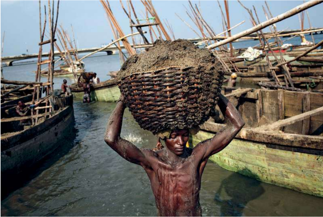
FIG 9.4 A sand miner in Nigeria carrying sand ashore from a boat filled with sand brought up by divers. Diving to mine sand from river bottoms is a dangerous mining technique that has resulted in a number of drownings. Photo ©Robin Hammond—Panos Pictures.
