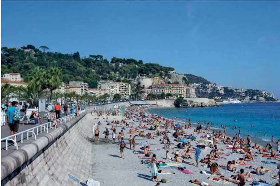
FIG 8.5 This pebble beach at Nice, France, is very steep. Every spring the beach is flattened to encourage tourism, and each year the portion of the beach that was extended seaward by bulldozers is lost to erosion. So, beach nourishment is an annual affair. Photo © kovog, Creative Commons CC BY-SA 2.0.
