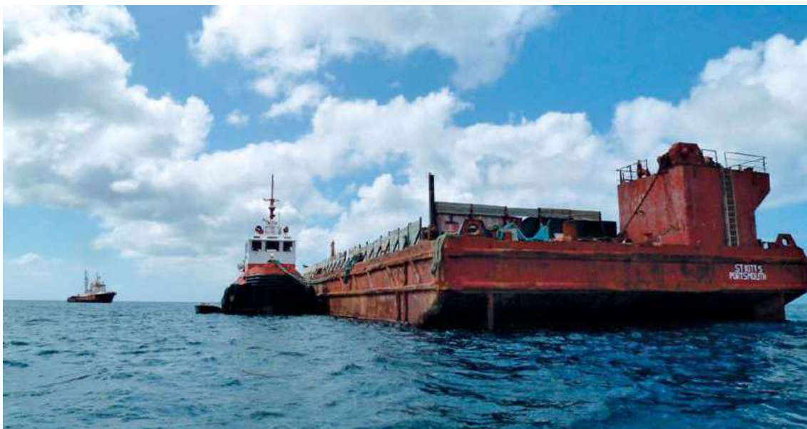
FIG 6.4 Sand-bearing barge off Grenada. The barge is not self-propelled but is guided by a tug. This common mode of transportation is used worldwide to transfer sand from one island to another including to Singapore from other countries or islands. Photo © SAF — Coastal Care.
