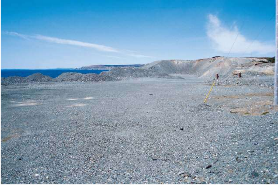
FIG 8.2 A featureless surface is all that remains from a mined-out gravel mine near Avalon, Newfoundland, Canada. Most Canadian beach mining takes place in rural areas and thus has limited impact on tourist beaches. Completely flattening the beach and dune, as has happened here, destroys the ecosystem and removes any storm-surge protection for roads or buildings adjacent to the beach. Photo © Joe Kelley.
