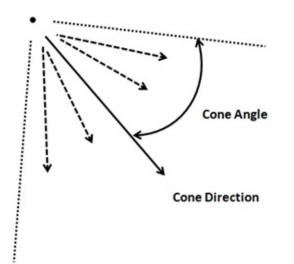
Spot light contribution is calculated in the same way as a point light with some exceptions. The point which the vector that points from the vertex position to the light source is not contained inside the light cone are not affected by the point light.
