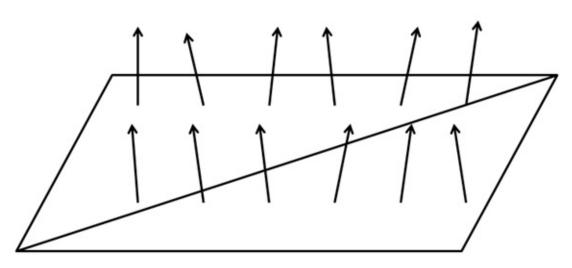
The way we are going to achieve this is by loading another texture which stores the normals for the surface. Each pixel of the normal texture will contain the values of the x, y and z coordinates of the normal stored as an RGB value.
