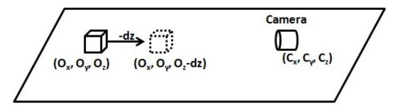
A camera can be displaced along the three axis (x, y and z) and also can rotate along them (roll, pitch and yaw).
