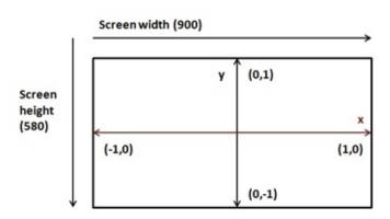
But, the problem is more serious than that. Modify the z coordinate of our quad from 0.0 to 1.0 and to -1.0. What do you see? The quad is exactly drawn in the same place no matter if it's displaced along the z axis. Why is this happening? Objects that are further away should be drawn smaller than objects that are closer. But we are drawing them with the same x and y coordinates.
