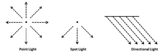
Thus, to model light we need to take into consideration the type of light plus, its position and some other parameters like its colour. Of course, we must also consider the way that objects, impacted by ray lights, absorb and reflect light.
