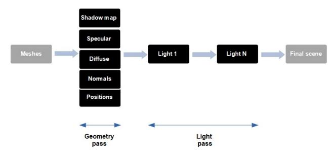
You may be asking if performing additional rendering passes will result in an increase of performance or not. The answer is that it depends. Deferred shading is usually used when you have many different light passes. In this case, the additional rendering steps are compensated by the reduction of operations that will be done in the fragment shader.
