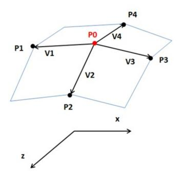
Then, we calculate the normal for each of the planes that connects the adjacent points. This is done by performing the cross product between the previous calculated vectors. For instance, the normal of the surface that connects P1 and P2 (shaded in blue) is calculated as the cross product between V1 and V2,  $V12 = V1 \times V2$ .
