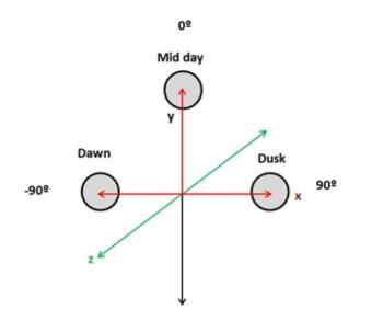
We need to update light direction so when the sun it's at dawn  $(-90^{\circ})$  its direction is (-1,0,0) and its x coordinate progressively increases from -1 to 0 and the "y" coordinate increases to 1 as it approaches mid day. Then the "x" coordinate increases to 1 and the "y" coordinates decreases to 0 again. This can be done by setting the x coordinate to the *sine* of the angle and y coordinate to the *cosine* of the angle.
