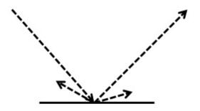
This is what the specular component models, and it depends on the material characteristics. Regarding specular reflectance, it's important to note that the reflected light will only be visible if the camera is in a proper position, that is, if it's in the area of where the reflected light is emitted.
