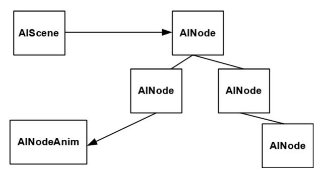
For a specific instant of time, for a frame, the transformation to be applied to a bone is the transformation defined in the animation channel for that instant, multiplied by the transformations of all the parent nodes up to the root node. Hence, we need to reorder the information stored in the scene, the process is as follows:
