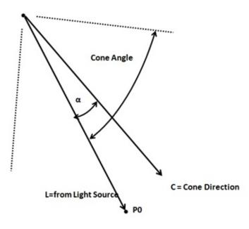
The dot product between L and C vectors is equal to:  $L \cdot C = |L| \cdot |C| \cdot Cos(\alpha)$ . If, in our spot light definition we store the cosine of the cutoff angle, if the dot product is higher than that value we will know that it is inside the light cone (recall the cosine graph, when  $\alpha$  angle is 0, the cosine will be 1, the smaller the angle the higher the cosine).
