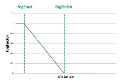
The linear model is easy to calculate but it is not very realistic and it does not take into consideration the fog density. In reality fog tends to grow in a smoother way. So the next suitable model is a exponential one. The equation for that model is as follows:
