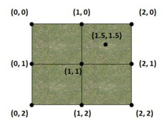
This is what we will do when setting the texture coordinates. We will be multiplying the texture coordinates (calculated as if the texture just was wrapped covering the whole mesh) by a factor, the textine parameter, to increase the number of pixels of the texture to be used between adjacent vertices.
