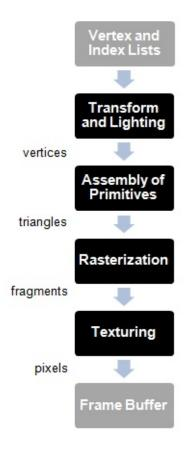
OpenGL 2.0 introduced the concept of programmable pipeline. In this model, the different steps that compose the graphics pipeline can be controlled or programmed by using a set of specific programs called shaders. The following picture depicts a simplified version of the OpenGL programmable pipeline:
