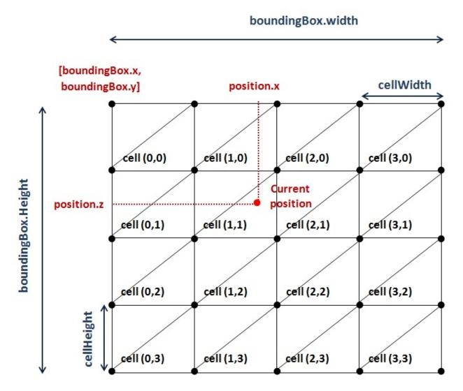
With all that information we are able to calculate the positions of the vertices of the triangles contained in the cell. How we can do this ? Let's examine the triangles that form a single cell.
