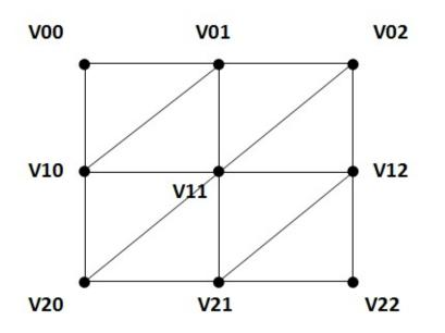
When we are processing the first vertex (V00), we define the indices of the two triangles shaded in red.
