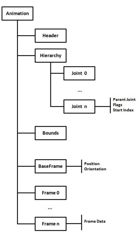
The first structure that you can find in the animation file, as in the case of the mesh definition file, is the header. You can see below header's content from one of the samples provided:
