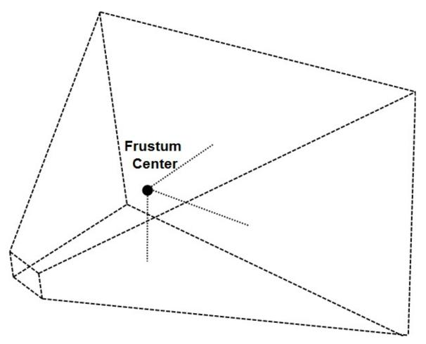
With that information we can set the position of the light. That position and its direction will be used to construct the light view matrix. In order to calculate the position, we start form the centre of the view frustum obtained before. We then go back to the direction of light an amount equal to the distance between the near and far z planes of the view frustum.
