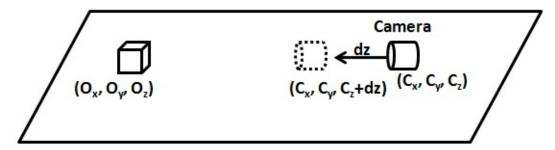
What we will actually do is move the object (all the objects in our 3D space indeed) in the opposite direction that the camera should move. Think about it like the objects being placed in a treadmill.
