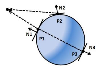
As you can see, the normal associated to P1, named N1, is parallel to the vector that points to the light source, which models the opposite of the light ray (N1 has been sketched displaced so you can see it, but it's equivalent mathematically). P1 has an angle equal to 0 with the vector that points to the light source. It's surface is perpendicular to the light source and P1 would be the brightest point.
