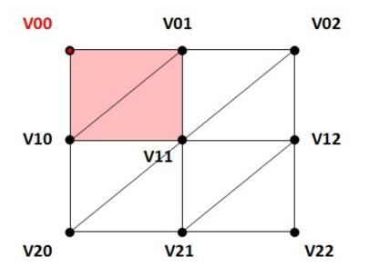
When we are processing the second vertex (V01), we define the indices of the two triangles shaded in red. But, when we are processing the the third vertex (V02) we do not need to define more indices, the triangles for that row have already been defined.
