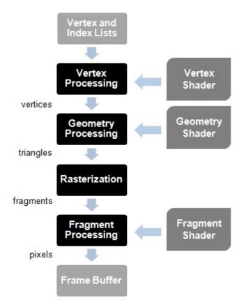
The rendering starts taking as its input a list of vertices in the form of Vertex Buffers. But, what is a vertex? A vertex is a data structure that describes a point in 2D or 3D space. And how do you describe a point in a 3D space? By specifying its x, y and z coordinates. And what is a Vertex Buffer? A Vertex Buffer is another data structure that packs all the vertices that need to be rendered, by using vertex arrays, and makes that information available to the shaders in the graphics pipeline.
