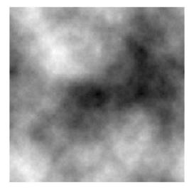
The image above it's like if you were looking at a fragment of land from above. With that image we will build a mesh composed by triangles formed by vertices. The altitude of each vertex will be calculated depending on the colour of each of the image pixels. Black colour will represent the lowest value and white the highest one.
