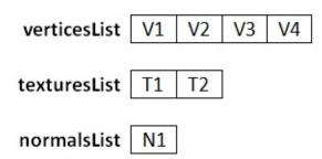
Now we will use the face definitions to construct the final arrays including the indices. A thing to take into consideration is that the order in which textures coordinates and vector normals are defined does not correspond to the orders in which vertices are defined. If the size of the lists would be the same and they were ordered, face definition lines would only just need to include a number per vertex.
