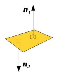
As you can see in the figure above a plane can have two normals, which one should we use ? Normals in 3D graphics are used for lightning, so we should chose the normal which is oriented towards the source of light. In other words we should choose the normal that points out from the external face of our model.
