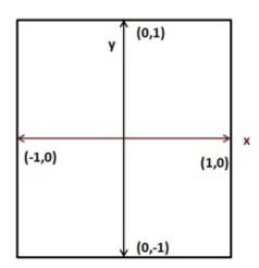
Those coordinates are mapped, considering our window size, to window coordinates (which have the origin at the top-left corner of the previous figure). So, if our window has a size of 900x480, OpenGL coordinates (1,0) will be mapped to coordinates (900, 0) creating a rectangle instead of a quad.
