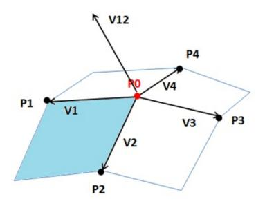
If we calculate the rest of the normals for the rest of the surfaces ( $V23 = V2 \times V3$ ,  $V34 = V3 \times V4$  and  $V41 = V4 \times V1$ ), the normal for P0 will be the sum (normalized) of all the normals of the surrounding surfaces:  $\hat{N0} = \hat{V12} + \hat{V23} + \hat{V34} + \hat{V41}$ .
