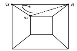
This is because, the skybox was defined to be looked from the outside. So we need to flip the definition of some of the faces in order to be viewed correctly when face culling is enabled.
