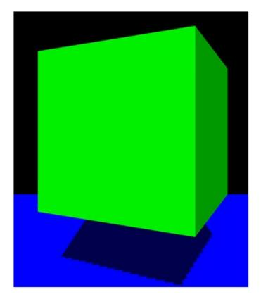
Now we are going to solve de shadow edges problem, which is also caused by the texture resolution. For each fragment we are going to sample the depth texture with the fragment's position value and the surrounding values. Then we will calculate the average and assign that value as the shadow value. In this case his value won't be 0 or 1 but can take values in between in order to get smoother edges.
