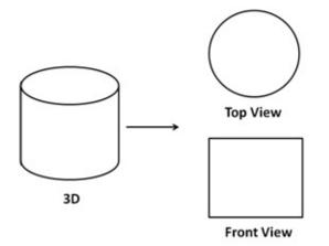
This projection is very convenient in order to draw 2D objects because it "ignores" the values of the z coordinates, that is, the distance to the view. With this projection the objects sizes do not decrease with the distance (as in the perspective projection). In order to project an object using an ortographic projection we will need to use another matrix, the orthographic matrix which formula is shown below.
