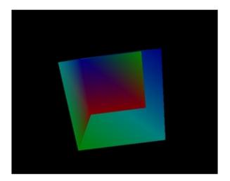
There is something weird with this cube. Some faces are not being painted correctly. What is happening? The reason why the cube has this aspect is that the triangles that compose the cube are being drawn in a sort of random order. The pixels that are far away should be drawn before pixels that are closer. This is not happening right now and in order to do that we must enable depth testing.
