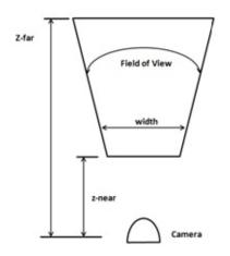
A projection matrix will correctly map 3D coordinates so they can be correctly represented on a 2D screen. The mathematical representation of that matrix is as follows (don't be scared).
