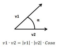
If both vectors are normalized, their length, their module will be equal to one, so the dot product is equal to the cosine if the angle between them. We will use that operation to calculate the diffuse reflectance component.
