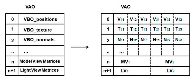
Thus, when rendering the first vertex of the first instance, V11, T11 and N11 would be used for position, texture and normal data and MV1 would be used as a model view matrix. When rendering the second vertex of the same first instance, V12, T12 and N12 would be used for position, texture and normal dara and MV1 wouls still be used as a model view matrix. MV2 and LV2 would not be used until second instance is rendered.
