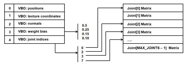
So, given a vertex position, we are calculating it's frame position as
