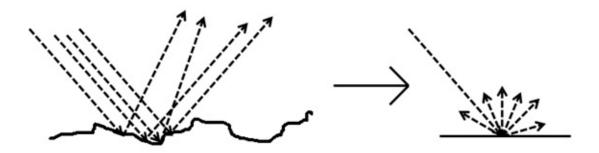
But when light impacts a polished surface, for instance a metal, the light suffers from lower diffusion and most of it gets reflected in the opposite direction as it hit that surface.
