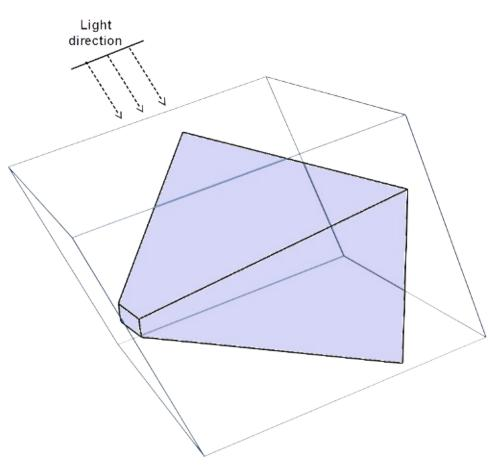
How can we construct that? The first step is to calculate the frustum corners of the view projection matrix. We get the coordinates in world space. Then we calculate the centre of that frustum. This can be calculating by adding the coordinates for all the corners and dividing the result by the number of corners.
