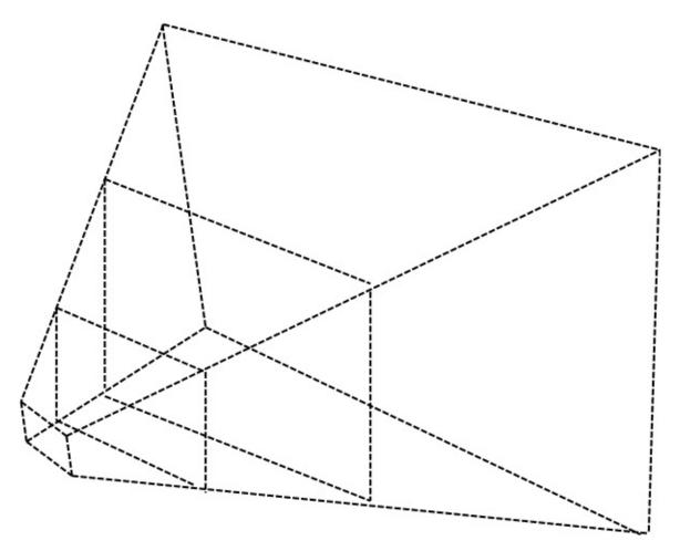
For each of these splits, the depth map is rendered, adjusting the light view and projection matrices to cover fit to each split. Thus, the texture that stores the depth map covers a reduced area of the view frustum. And, since the split closest to the camera covers less space, the depth resolution is increased.
