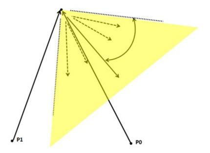
How do we calculate if it's inside the light cone or not ? We need to do a dot product again between the vector that points from the light source and the cone direction vector (both of them normalized).
