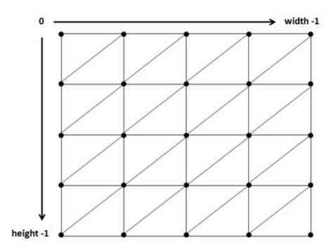
That mesh will form a giant quad that will be rendered across x and z axis using the pixel colours to change the elevation in the y axis.
