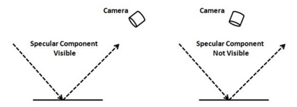
Once the mechanism that's behind sepecular reflection has been explained we are ready to calculate that component. First we need a vector that points from the light source to the vertex point. When we were calculating the difusse component we calculated just the opposite, a vector that points to the light source. toLightDirection, so let's calculate it as fromLightDirection = -(toLightDirection).
