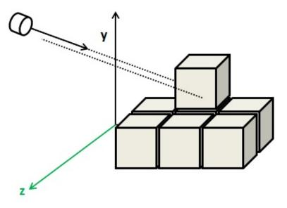
We have the camera, placed in some coordinates in world-space, facing a specific direction. Any object that intersects with a ray cast from camera's position following camera's forward direction will be a candidate. Between all the candidates we just need to chose the closest one.
