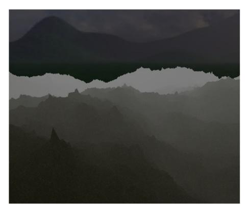
Distant objects are set to the fog colour which is a constant and not affected by light. This fact produces like a glowing in the dark effect (which may be ok for you or not). We need to change the function that calculates the fog to take into consideration the light. The function will receive the ambient light and the directional light to modulate the fog colour.
