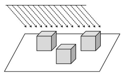
Another characteristic of directional light is that it is not affected by attenuation. Think again about Sun light, all objects that are hit by ray lights are illuminated with the same intensity, the distance from the sun is so huge that the position of the objects is irrelevant. In fact, directional lights are modeled as light sources placed at the infinity, if it was affected by attenuation it would have no effect in any object (it's colour contribution would be equal to 0).
