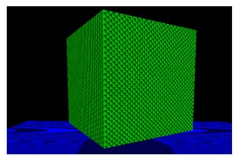
Although shadows are working (you can check that by moving light direction), the implementation presents some problems. First of all, there are strange lines in the objects that are lightened up. This effect is called shadow acne, and it's produced by the limited
