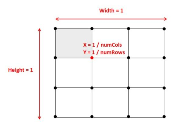
Then we just need to apply and offset depending on the row and column, this is what is modelled by the texxoffset and texyoffset uniforms.
