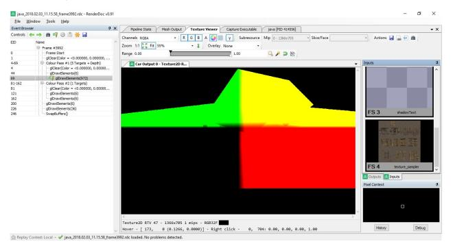
In the center panel, you can see the output, and on the right panel you can see the list of textures used as an input. You can also view the output textures one by one. This is very illustrative to show how deferred shading works.
