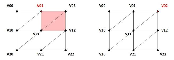
You can easily see how the process continues for the rest of vertices. Now, once we have created all the vertices positions, the texture coordinates and the indices we just need to create a Mesh and the associated Material with all that data.
