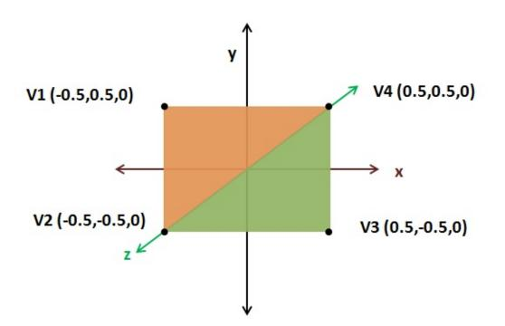
As you can see each of the two triangles is composed of three vertices. The first one formed by the vertices V1, V2 and V4 (the orange one) and the second one formed by the vertices V4, V2 and V3 (the green one). Vertices are specified in a counter-clockwise order, so the float array to be passed will be [V1, V2, V4, V4, V2, V3]. Thus, the init method in our DummyGame class will be:
