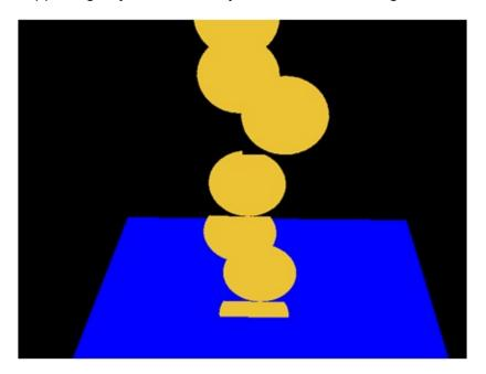
Why some particles seem to be cut off? Why the transparent background does not solve this? The reason for that is depth testing. Some fragments of the particles get discarded because they have a depth buffer value higher than the current value of the depth buffer for that zone. We can solve this by ordering the particle drawings depending in their distance to the camera or we can just disable the depth writing.
