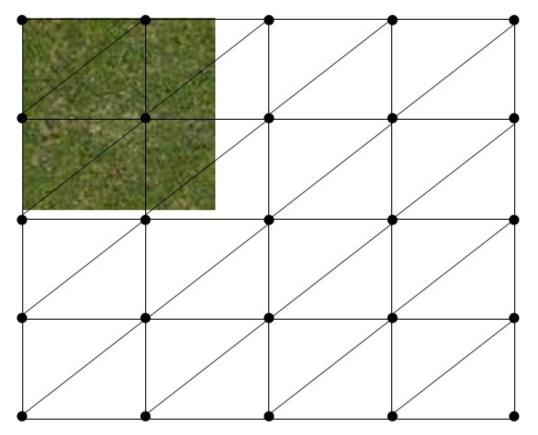
The only thing that's pending now is normal calculation. Remember that we need normals so light can be applied to the terrain correctly. Without normals our terrain will be rendered with the same colour no matter how light hits each point. The method that we will use here may not be the most efficient for height maps but it will help you understand how normals can be auto-calculated. If you search for other solutions you may find more efficient approaches that
