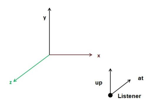
The "at" vector basically points where the listener is facing, by default its coordinates are (0,0,-1). The "up" vector determines which direction is up for the listener and, by default it points to (0,1,0). So the tree components of each of those two vectors are what are set in the alListenerfy method call. This method is used to transfer a set of floats (a variable number of floats) to a property, in this case, the orientation.
