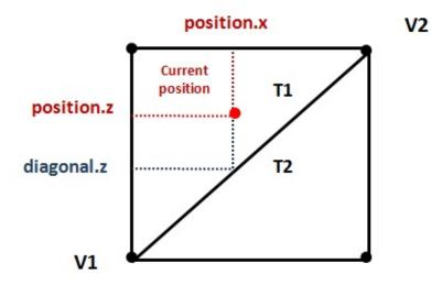
You can see that the cell is divided by a diagonal that separates the two triangles. The way to determine the triangle associated to the current position, is by checking if the z coordinate is above or below that diagonal. In our case, if current position z value is less than the z
