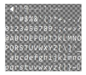
As you can see, the image has all the characters displayed in rows and columns. In this case the image is composed by 15 columns and 17 rows. By using the character code of a specific letter we can calculate the row and the column that is enclosed in the image. The
