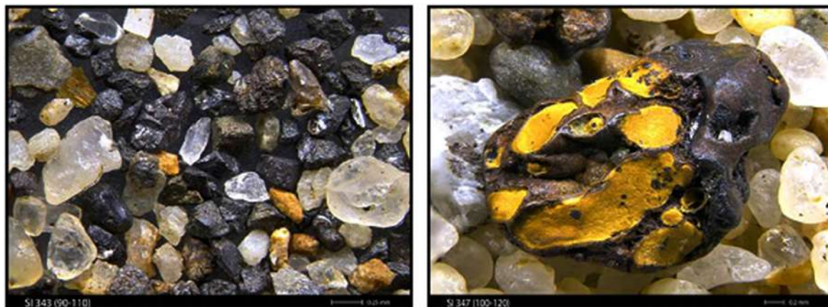
FIGURE 10 | View under stereo microscope of sediment. Mining residues in the sediments (ISPRA, 2015).
