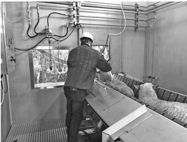
Figure 12.6 Head to back electrical stunner being used on sheep. This device simultaneously passes the electric current through the brain and the heart to produce both instantaneous unconsciousness and cardiac arrest. The sheep are riding to the stunning a V-conveyor restrainer (photo credit: Temple Grandin).
