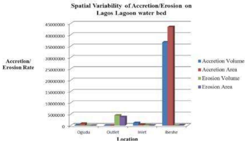
**Figure 19.** Chart showing spatial variability of sediment accretion and erosion on Lagos Lagoon bed based on two repeated bathymetric data of 2008 and 2014. Area = metres squared and volume = metres cubed.
