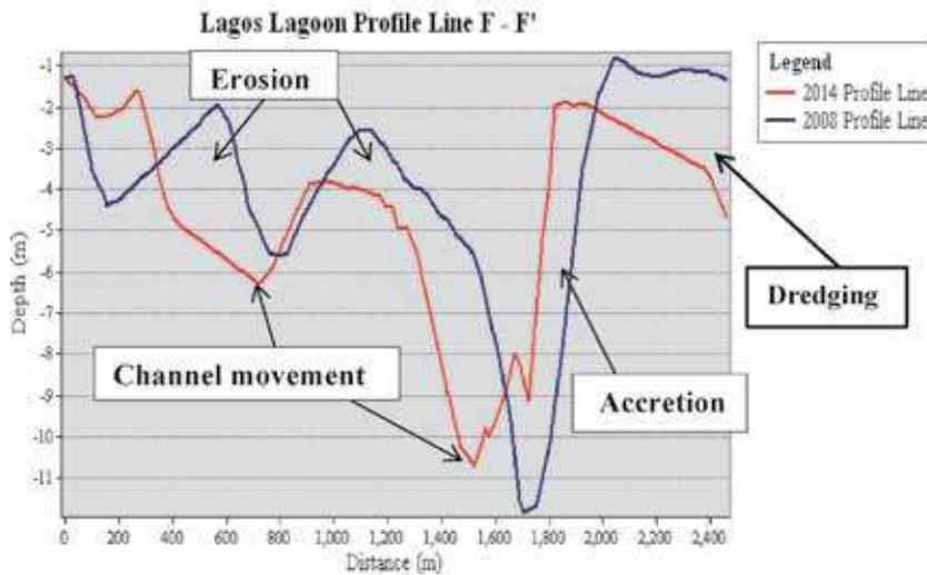
**Figure 9.** Profile section F-F' showing trend of variation in the repeated bathymetric data.
