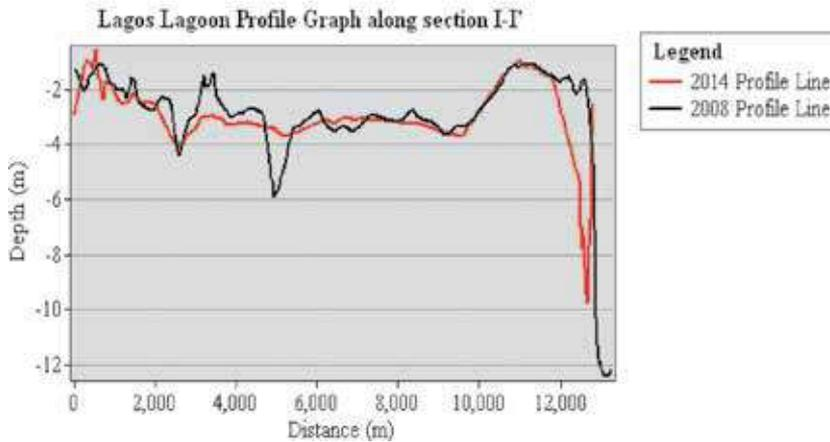
**Figure 16.** Profile section I-I' showing degree of variation in the depths of the lagoon repeated bathymetric data.
