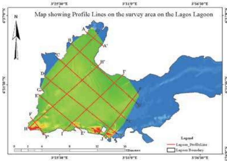
**Figure 3.** Lagos Lagoon with profile lines on the study area. The area on the map with colour blue indicates area covered by the bathymetric survey of 2008, while the area with greenish yellow colour shows area surveyed in 2014.
