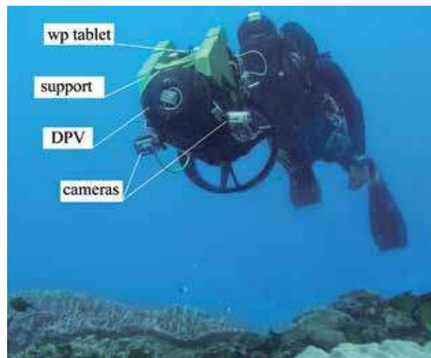
**Figure 5.** The driver propulsion system (DPV), a remotely operated vehicle (ROV), equipped with a waterproof (wp) tablet and cameras. The tablet is used to coordinate data collection and steer vehicle direction.
