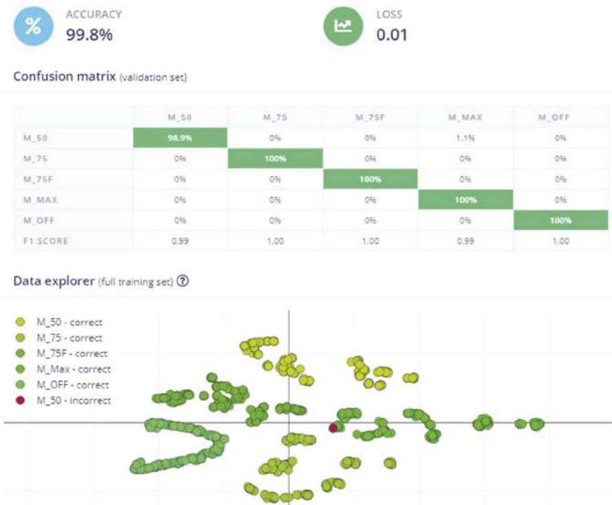
Figure 12.6 Confusion Matrix and Data Explorer based on full training set: Correctly Classified (Green) and Misclassified (Red).
