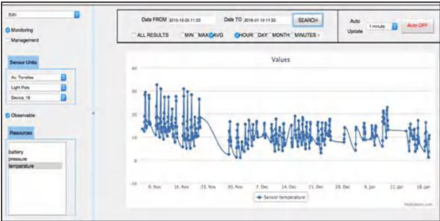
Figure 7.12 Temperature measurements captured by a low power wake-up device in Sant Vicenç dels Horts.
