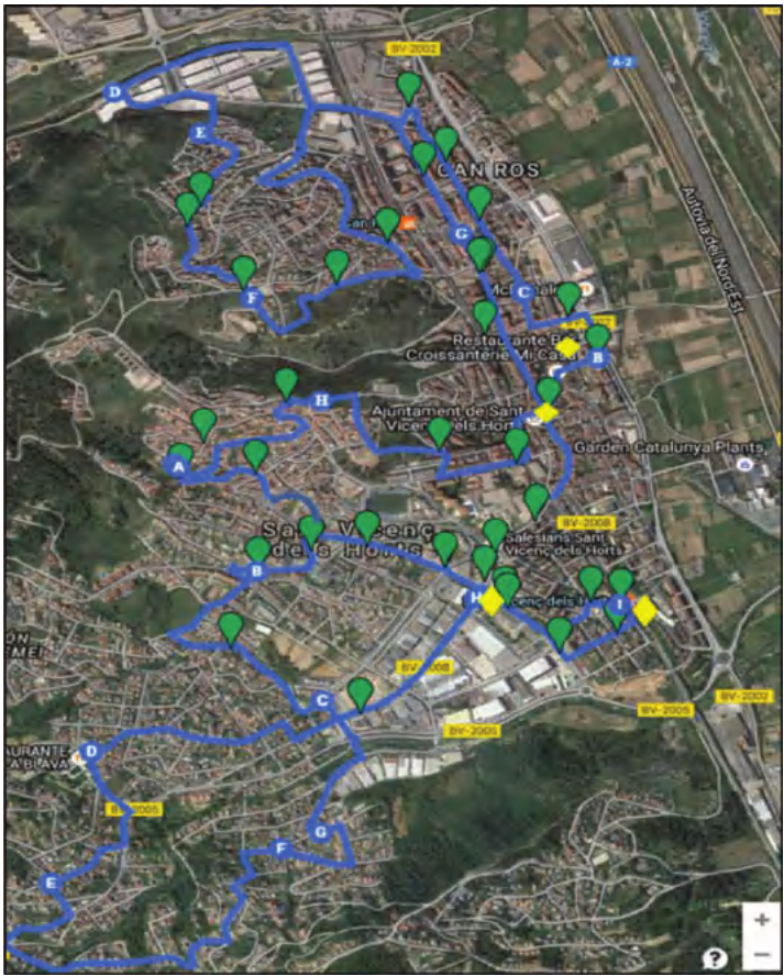
Figure 7.9 Routes followed by the bus and location of the sensor units: low-power wake-up (green) and Airbase air quality (yellow) devices.
