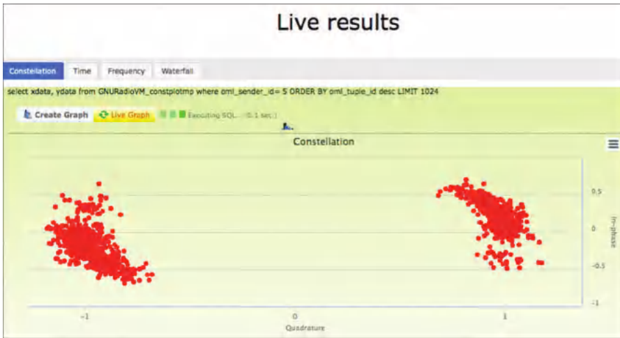
Figure 17.22 Real-time constellation measurements.
