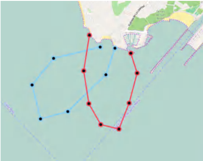
Figure 15.7 Waypoints definition for two USVs.
