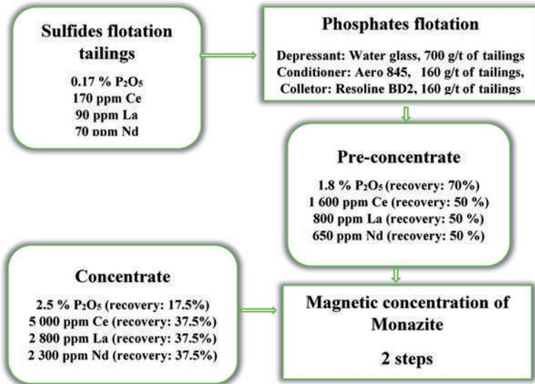
Fig. 2 Proposed process scheme for the beneficiation of REE in the flotation tailings from New Kankberg mine. (Adopted from [28])
