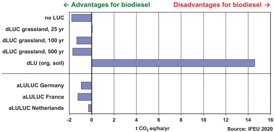
**Fig. 1** Life cycle greenhouse gas emissions of European rapeseed biodiesel compared to conventional diesel. All results are based on the same life cycle comparison with differences only in the used land and the methodological approach to land use (LU) and land use change (LUC). The time horizons, over which one-time emissions are distributed, are specified where applicable
