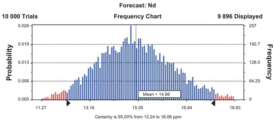
Fig. 5 CB forecast chart: Nd after 10,000 trials (95% confidence interval). Certainty is 95.00% from 12.24 to 18.06 ppm. (Source: own work)
