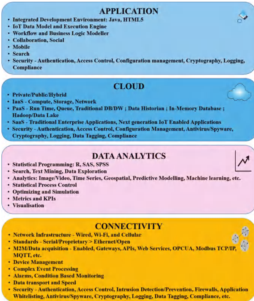
Figure 3.33 Implementation elements in the main areas covered by IoT platforms [14].
