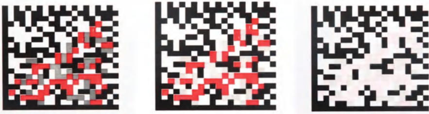
Figure 9.10 Data Matrix code with two functional inks. Code size is 3 cm x 3 cm. In the left picture both thermochromic inks can be seen ( T < +31^{\circ}\text{C} ). In the middle picture black thermochromic ink has disappeared ( +31^{\circ}\text{C} < T < +47^{\circ}\text{C} ). In the right picture both black and red thermochromic inks have disappeared ( T > +47^{\circ}\text{C} ).
