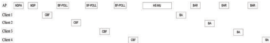
Figure 12.8 Downlink MU TXOP for 11ac.
