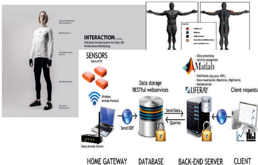
Figure 13.3 The different components of the Interaction monitoring system ( https://www.xsens.com/news/interaction-project/ ).
