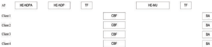
Figure 12.9 Downlink and uplink MU for 11ax.
