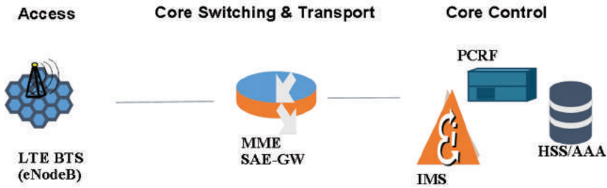
Figure 10.6 LTE/SAE system architecture (Picture NSN).
