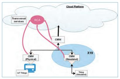
Figure 10.10. RCA - Rail Use Case integration synoptic.
