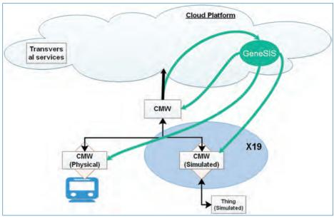
**Figure 10.6.** GeneSIS – Rail Use Case integration synoptic. *Source*: INDRA.
