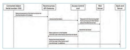
Figure 7.20. Context-aware Access Control with WAM as reverse-proxy — Sequence diagram.
