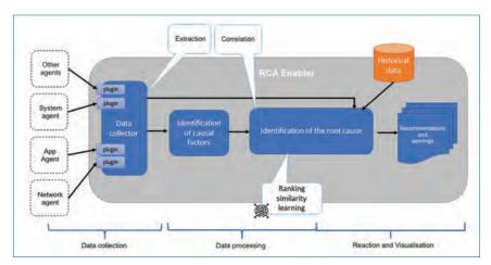
Figure 8.22. RCA Enabler high level architecture.
