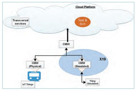
**Figure 10.7.** Testing and Simulation – Rail Use Case integration synoptic. *Source*: INDRA.
