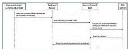
**Figure 7.21.** Context-aware Access Control with WAM as OpenID Connect IDP – Sequence diagram.
