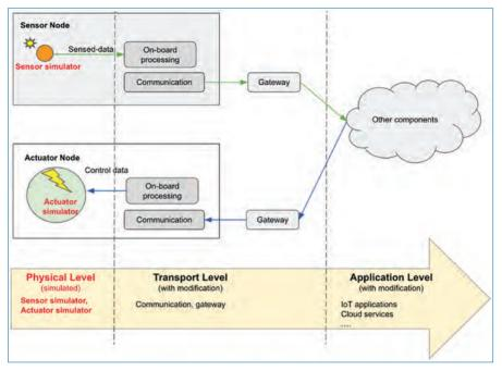
Figure 8.2. An IoT network architecture with simulated components.
