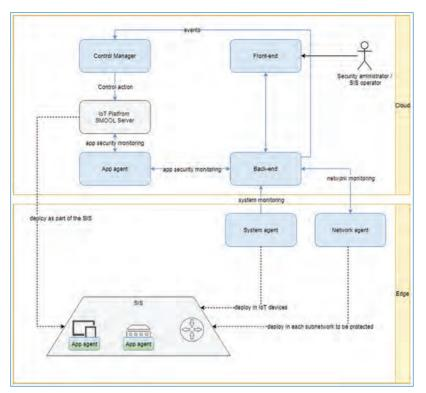
**Figure 7.13.** Architecture of the the Security and Privacy Monitoring and Control Enabler integrated with SMOOL IoT Platform.
